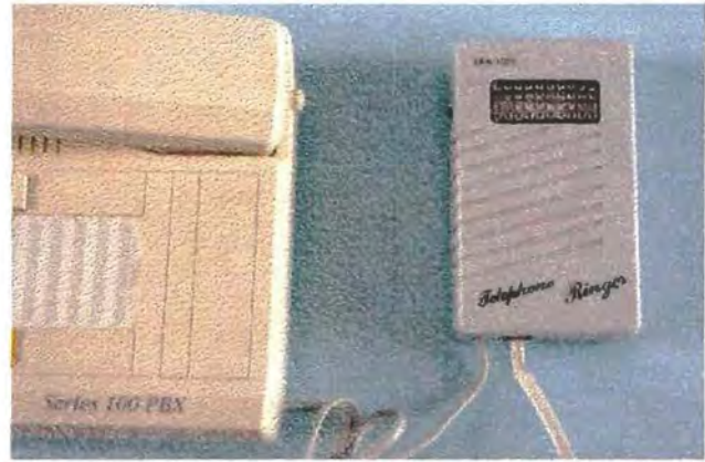
Telephone ringer with flasher (Telkom)
