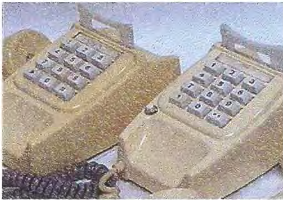
Lorea – 1981 The new electronic model is on the left – characterised by the “star” and “hash” symbols
