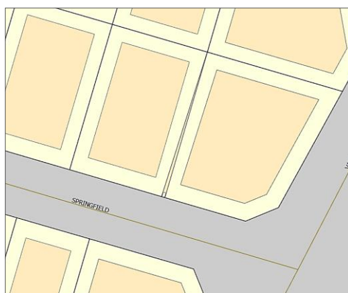
Figure 6-3: An example of a topological error in the land parcel dataset – a sliver is clearly visible between two land parcels.
