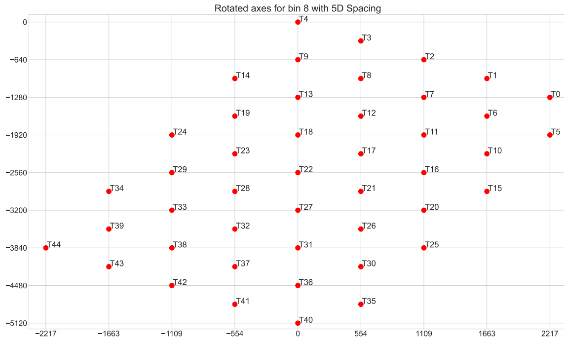
Figure 12: Wind plant array with 5D minimum T-2-T distance, Bin 8
