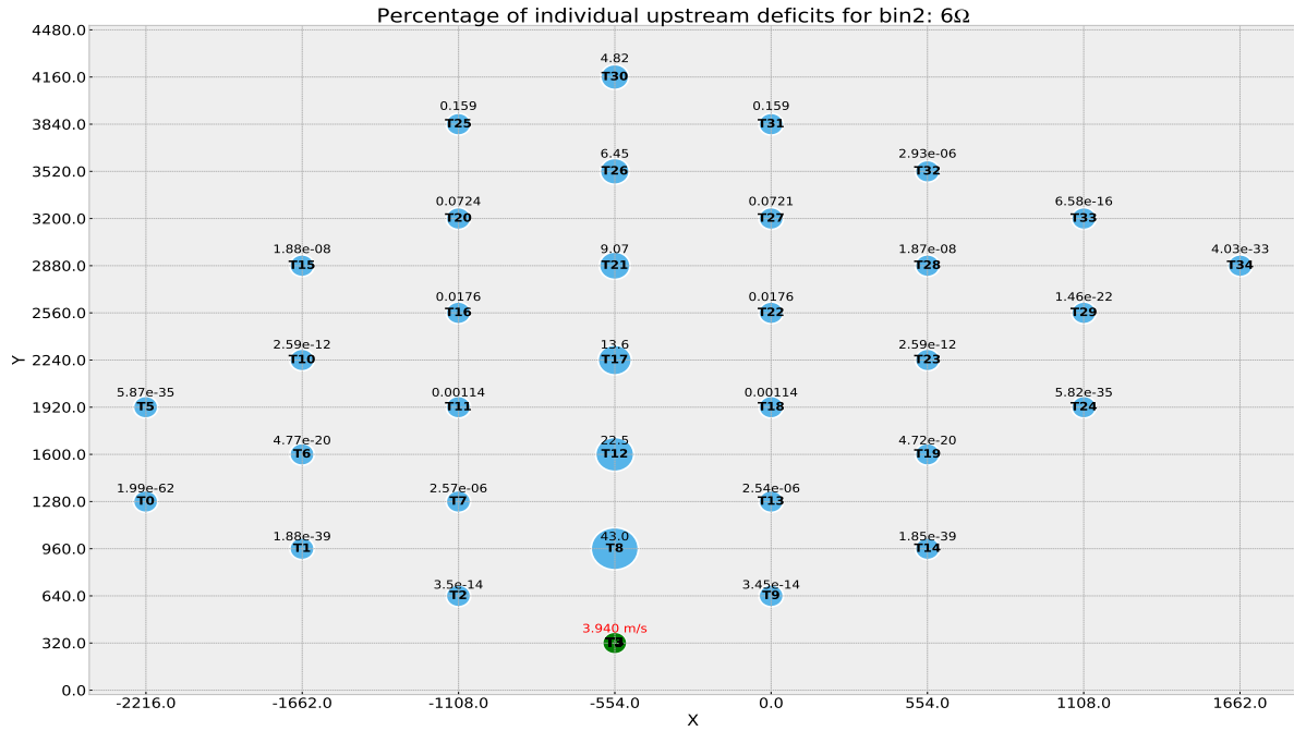
Figure 65: Percentage deficits from turbines within a 6\Omega upstream sector of T_3 ; Bin 2
