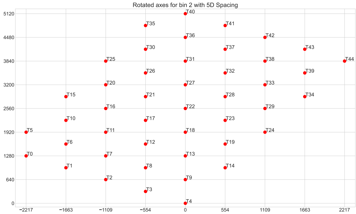
Figure 6: Wind plant array with 5D minimum T-2-T distance, Bin 2
