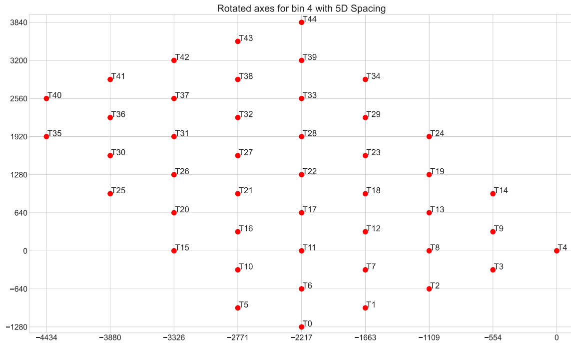
Figure 8: Wind plant array with 5D minimum T-2-T distance, Bin 4
