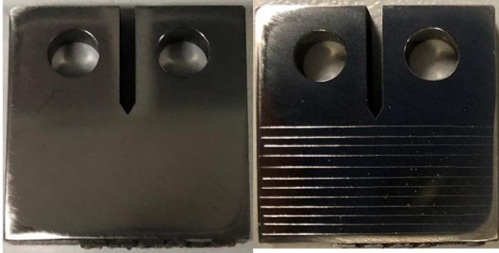
Figure 49: Fatigue crack growth rate specimen before testing. image on the right is the same specimen with scribes about 1 mm apart to monitor crack propagation
