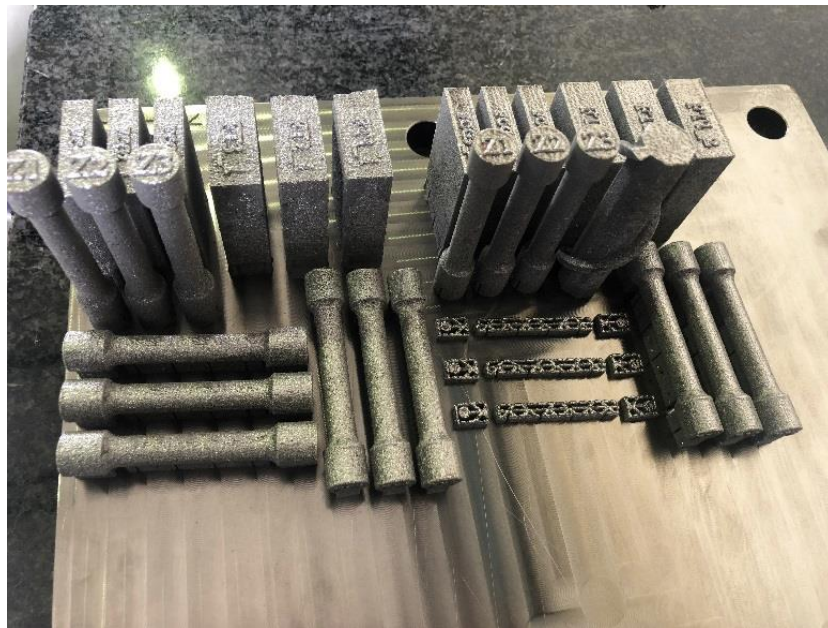
Figure 43: Specimens built for microstructure analysis and mechanical testing at the CSIR National Laser Centre
