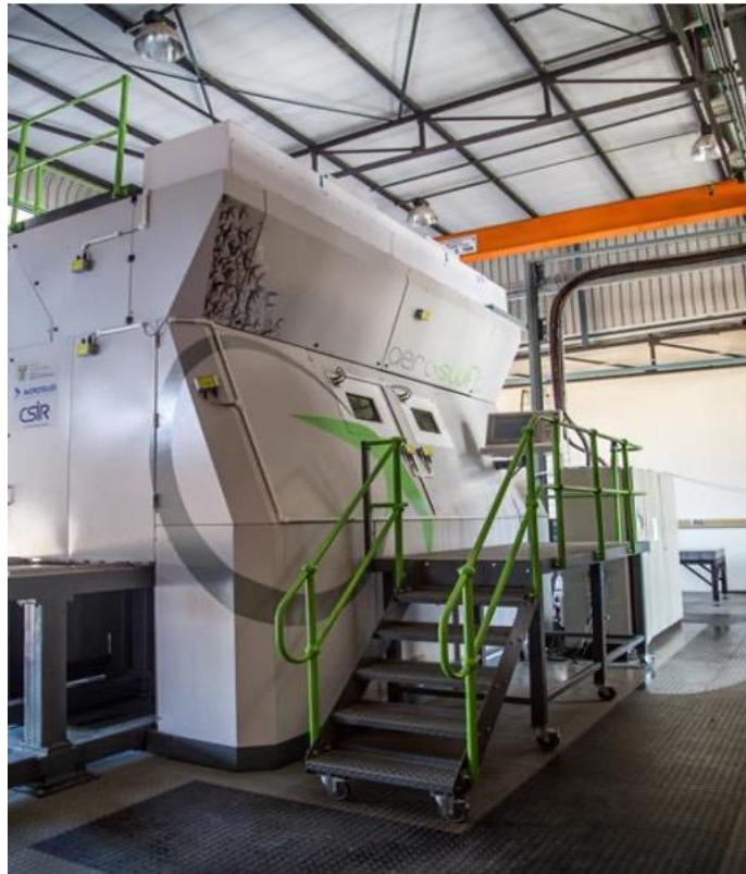
Figure 42: The Aeroswift machine used to build the SLM samples at the CSIR National Laser Centre.
