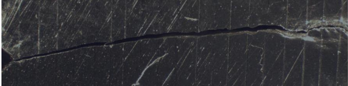
Figure 105: Fatigue crack for 6.5 m/s specimen 1
