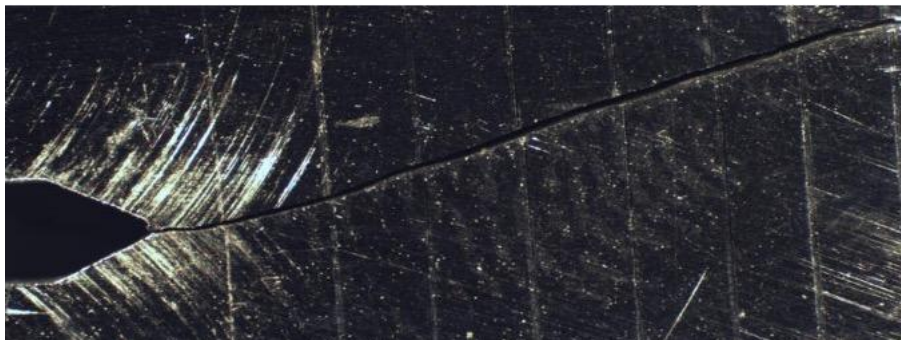
Figure 96: Fatigue crack path deviating from the horizontal
