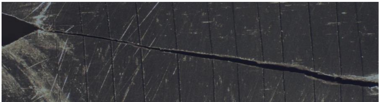
Figure 104: Fatigue crack for 6.25 m/s specimen 2
