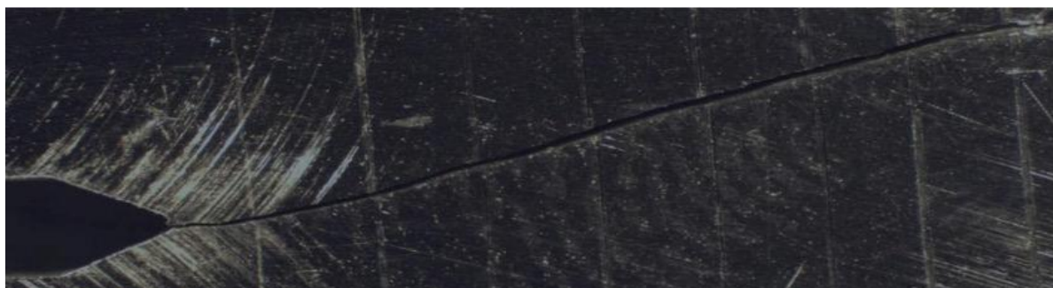
Figure 98: Fatigue crack for 5.5 m/s specimen 1
