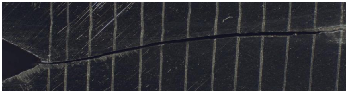
Figure 107: Fatigue crack for 6.5 m/s specimen
