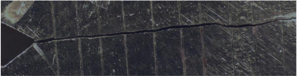
Figure 100: Fatigue crack for 6.0 m/s specimen 1
