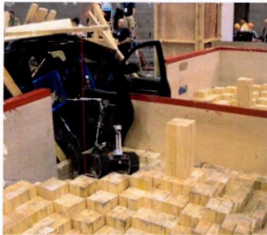
Figure 2.5.: A rescue robot inspecting a car in the black arena [10].
