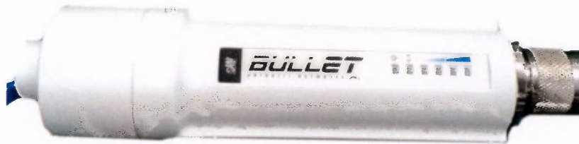
Figure 8.7.: A Ubiquiti Bullet M5 wireless radio.
