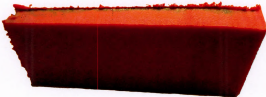
Figure 7.11.: The smooth surface as a result of a TPU component being cut by a band saw.
