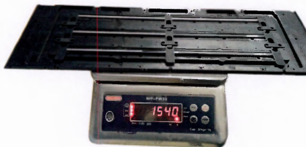
Figure 9.1.: The assembled top plate of the right sidepod being weighed.
