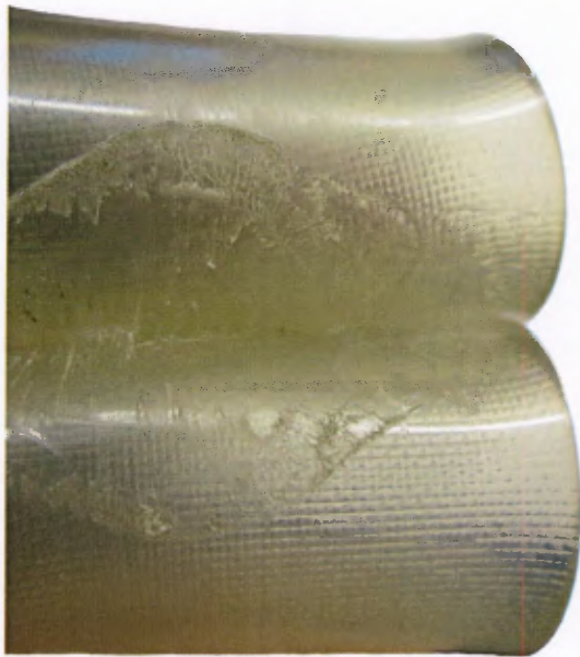
(a) The tearing that can be seen on the surface is an indication of successful bonding.
