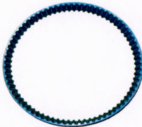
Figure 7.3.: One of the four flipper tracks in the previous development of the track system.
