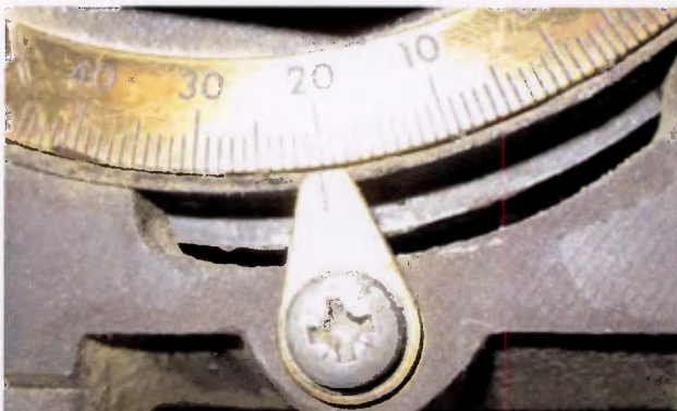
(a) the band saw's dial is set to 20^\circ .
