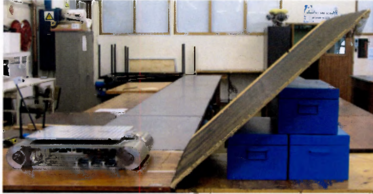
Figure 9.43.: The initial inclined plane climbing test.
