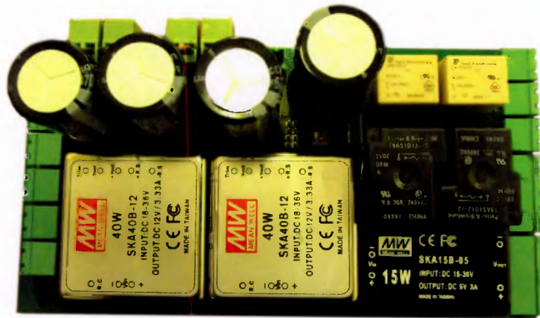
Figure 5.4.: The previous power distribution board developed by Eugene Dreyer.
