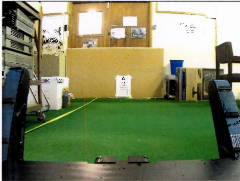
Figure 9.21.: A normal snapshot of the HD camera viewing the Snellen chart at a distance of 4.94m.
