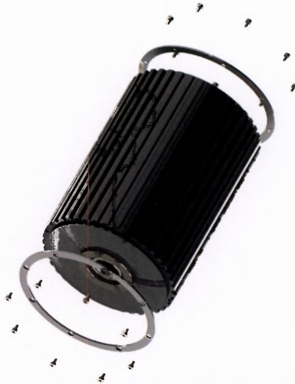
(a) A Solidworks render of one of the rear pulleys.
