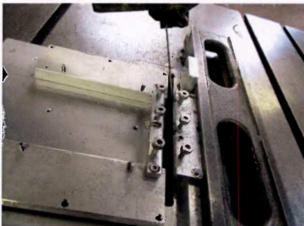
(a) Cutting jig on the band saw table.
