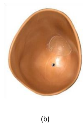
Figure 2.4: Socket Types: (a) Patella Tendon Bearing (PTB) socket, which contains features for concentrating large pressures onto pressure tolerant areas (Patella Tendon Bar). (b) Total Surface Bearing (TSB) socket, which distributes the load equally over the residual limb (Barnard, 2017).
