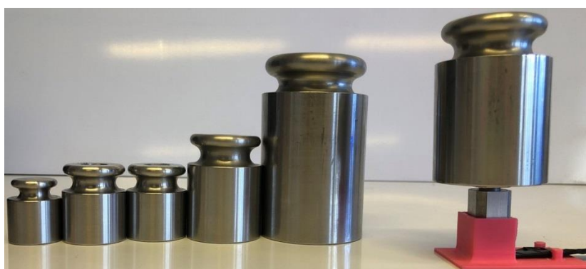
Figure 4.4: Weight application for calibration of pressure sensors.
