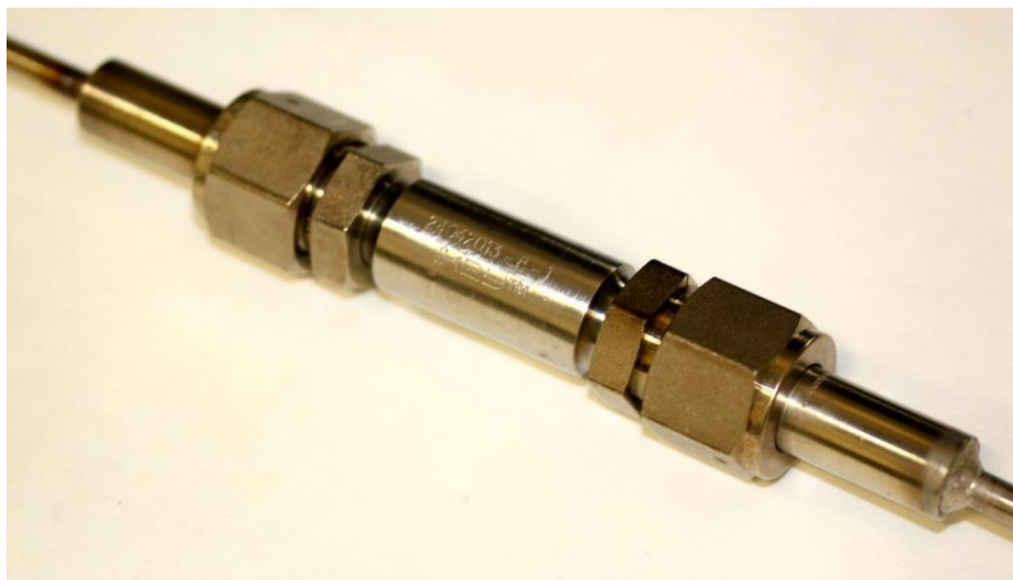
Figure 2.2: Reactor used for preparation of chemical deposition catalysts [6] .
