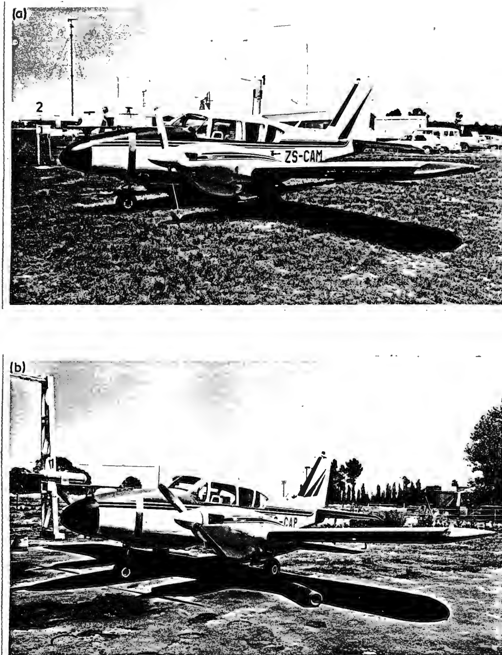
Fig. 3.7 The Aztec observation aircraft, (a) CAM, which is equipped with a 1) Mee Model 101 ice particle replicator, 2) PMS one dimensional optical array cloud droplet spectrometer, and (b) CAP, which is fitted with 1) PMS forward scattering spectrometer probe.
