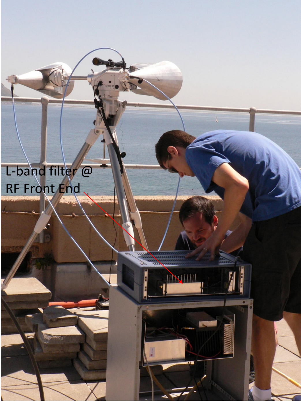
Figure 1.2: L and X-band filters being used at the RF front end of NeXtRAD at the test site: Simon’s Town (RSA)
