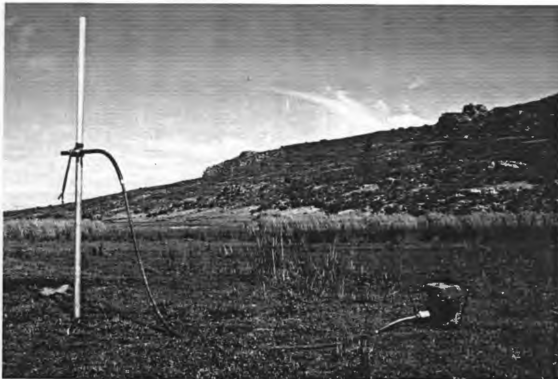
Plate 5.1. The assembled Vibracorer (Note the poker vibrator attached to the aluminium tube by means of pneumatic cable).
