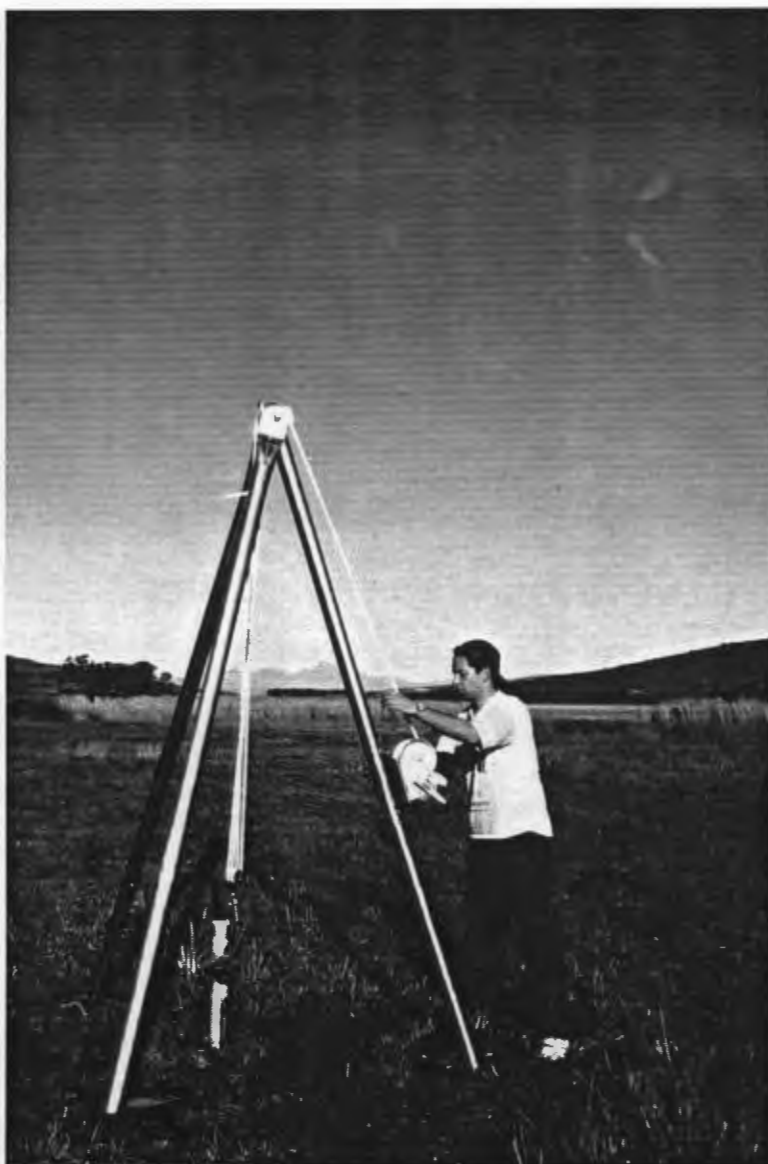
Plate 5.4. Extraction of the core tube by means of a tripod and pulley.
