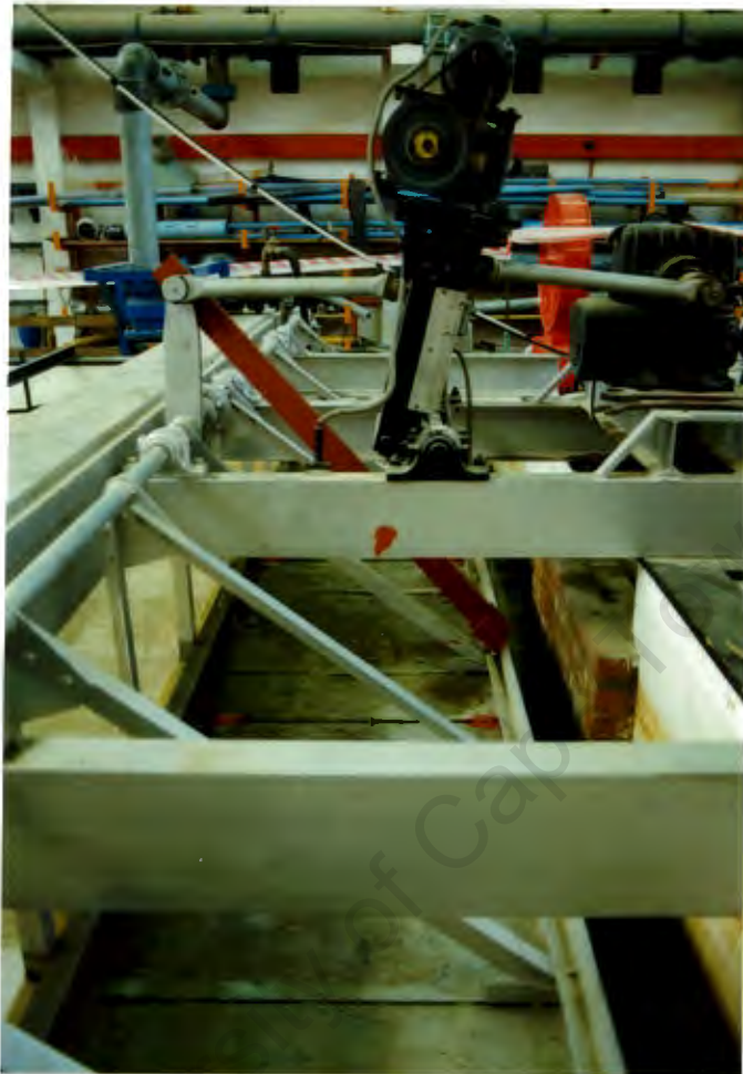
Plate 5.5 Modifications to the wave paddle
