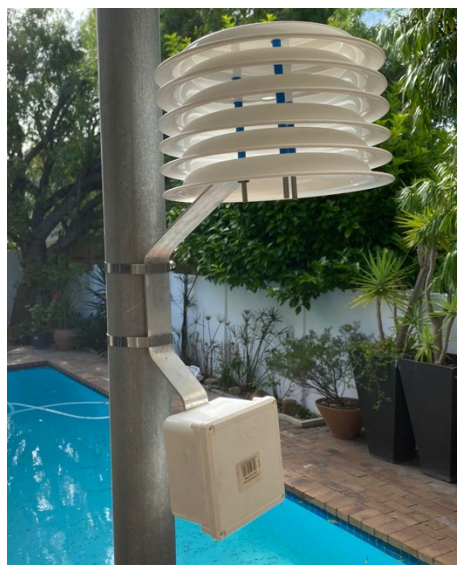
Figure 3-14: Bracket and solar radiation shield
