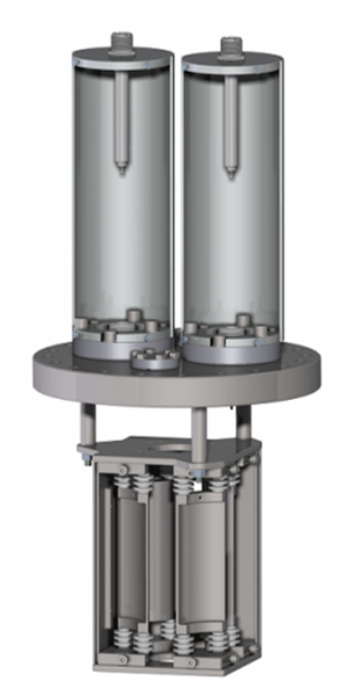
Figure 4.20: Image of the switch-yard from the Dre-EBIT website [30]. The vacuum chamber is shown at the bottom with the four electrodes which are powered with opposite biases up to \pm 25 kV. The two power supplies and their protective casings are connected above the switch-yard.
