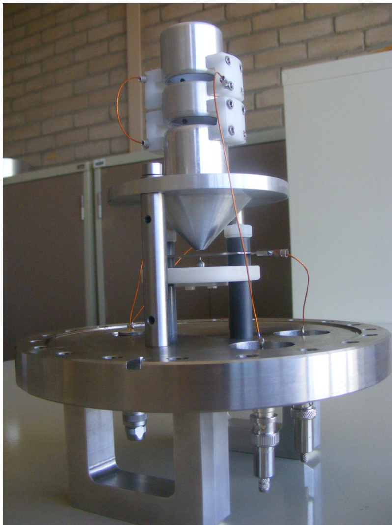
Figure 4.13: Photograph of the first LMIS ion extraction and focusing assembly. The LMIS unit is held in place securely and focused on axis. A high positive potential on the LMIS and a high negative potential on the nearby extraction plate provide a strong electric field around 100 \text{ V/nm} which causes field evaporation and metallic ion formation. The ion beam is then shaped and focused by a grounded conical electrode followed by einzel lenses.
