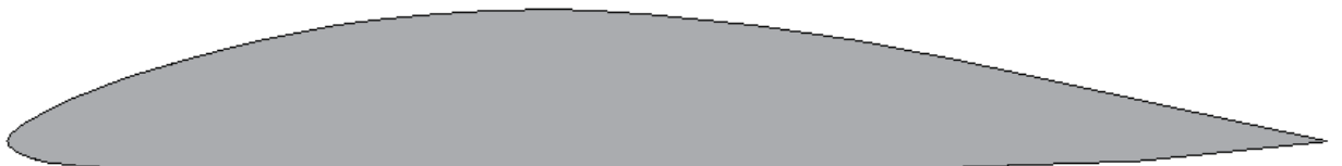
Figure 24: Profile shape of the DHMTU 10-40-2-10-2-60-21-5 aerofoil [4]
