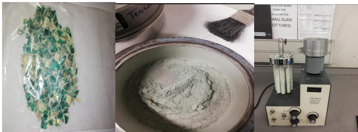
Figure 3-3: (a) Shredded PCB (b) PCB powder product after Pulverisation (c) Splitting process.
