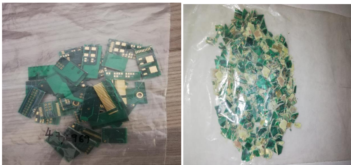
Figure 3-7:(a) PCBs cut into 3cm x 2cm Pieces
