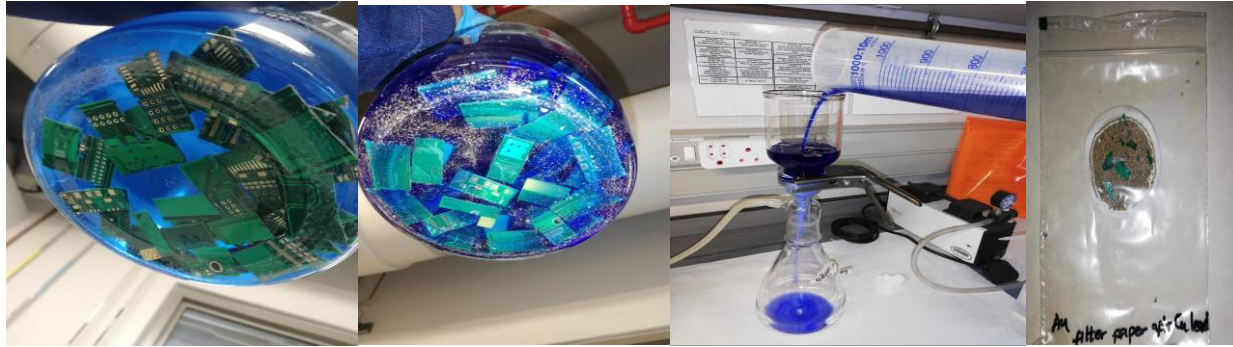
Figure 4-5: (a) Reactor at time t=0 hours (b) Au flakes t=72 hours (c) filtration of the flakes (d) filtered flakes
