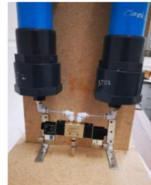
Sieve Beds Connected to a 5/2 12V solenoid Valve and 8mm snap on fittings
