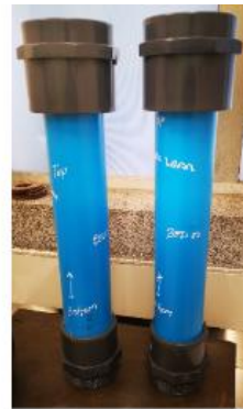
PVC Sieve beds Made from Class 16 Pipes and Class 32 Effast Fittings
