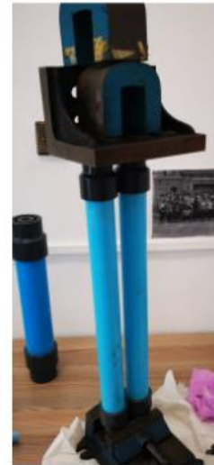
Top Sealed with an end cap and PVC cement. Weights are put on top to compress spring loaded sieve cap.
