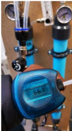
Testing was done using an external 1.5 Hp compressor at the flow rate of 5Lpm
