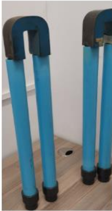
fabrication of the Zeolite Beds.
