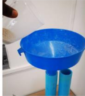
Filling Sieve Canisters with dry Zeolite Granules
