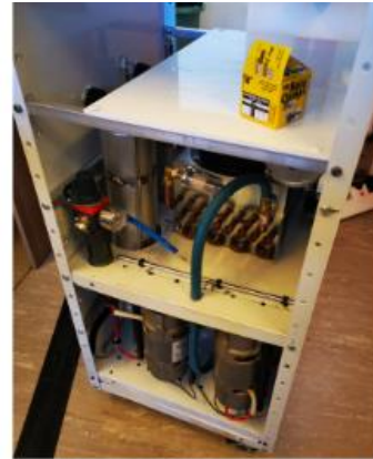
Assembled Air Cooler and Air pumps
