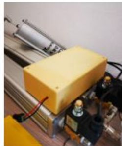
Connect 3/2 Solenoid Valves and test
