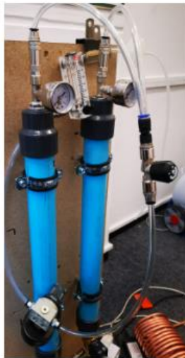
Prototype #2 fully assembled and fitted with a Copper Cooling Coil.
