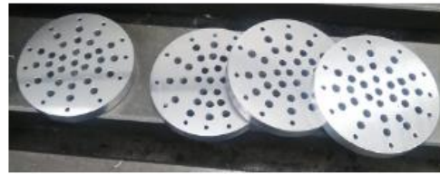
Spacer to separate Sieve molecules from the end-cap
