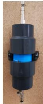
Oxygen Tank made of 75mm PVC class 16 Pipe and Class 32 endcaps glued together using a PVC cement
