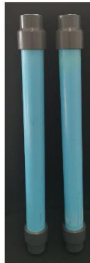
Canisters fully compressed and endcaps cemented.
