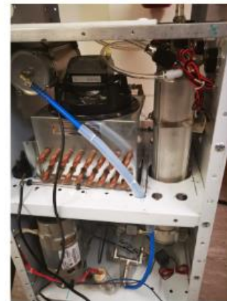
Assembled unit showing an air Buffer tank
