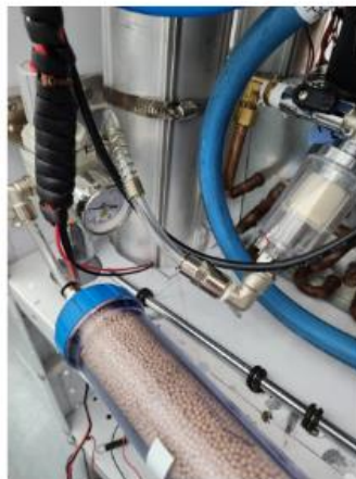
assembly showing a mechanical air dryer and a molecular activated alumina zeolite dryer.
