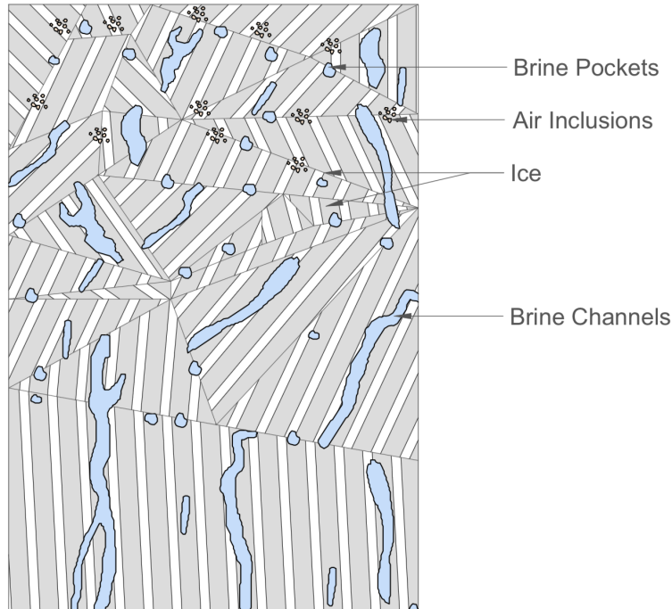
Figure 2.8. Schematic depicting the multiphase composition of sea ice made up of a porous solid (ice), liquid (brine) and gas (air).
