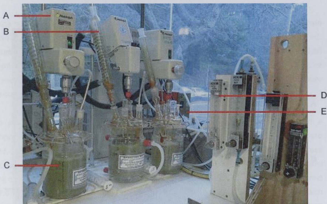
A- overhead stirrer, B- condenser, C- STR, D- air flow meter, E- water bath
