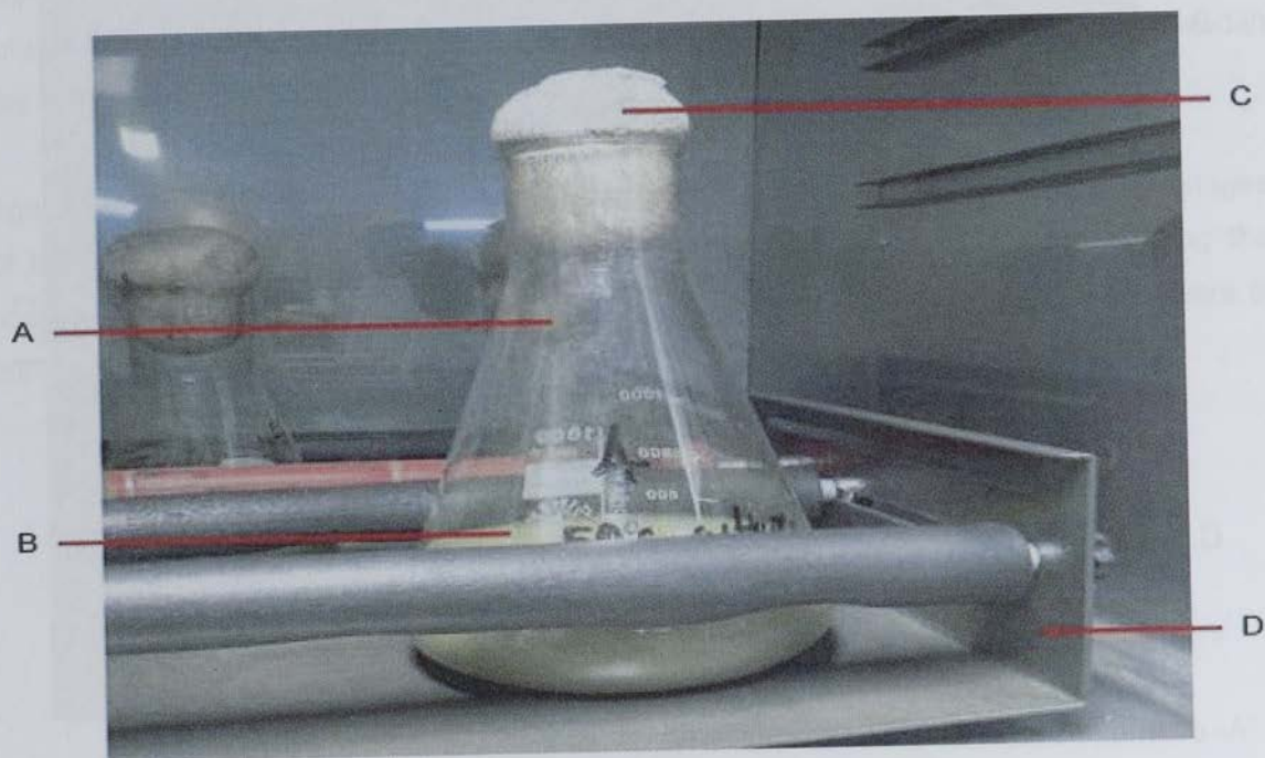
A- Erlenmeyer flask, B- culture, C- cotton wool plug, D- shaking platform
