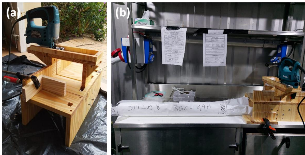
Figure 2.9. (a) wooden ice core cutting rig with jigsaw, (b) cutting set up in the polar laboratory.
