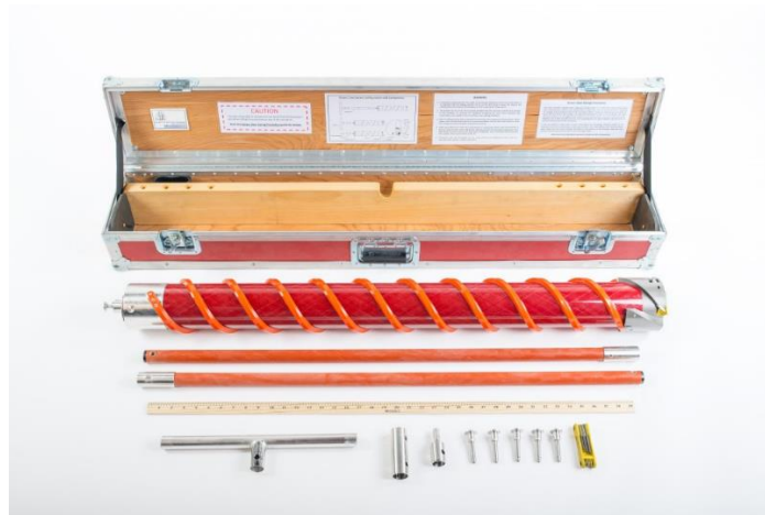
Figure 2.7. The Kovacs Mark II sea ice coring system used sea-ice floe during both SCALE2019 cruises. The barrel can retrieve a core up to 1 m long and 9 cm in diameter. Image retrieved from the Kovacs website ( https://kovacsicedrillingequipment.com/coring-systems/mark-ii/ )
