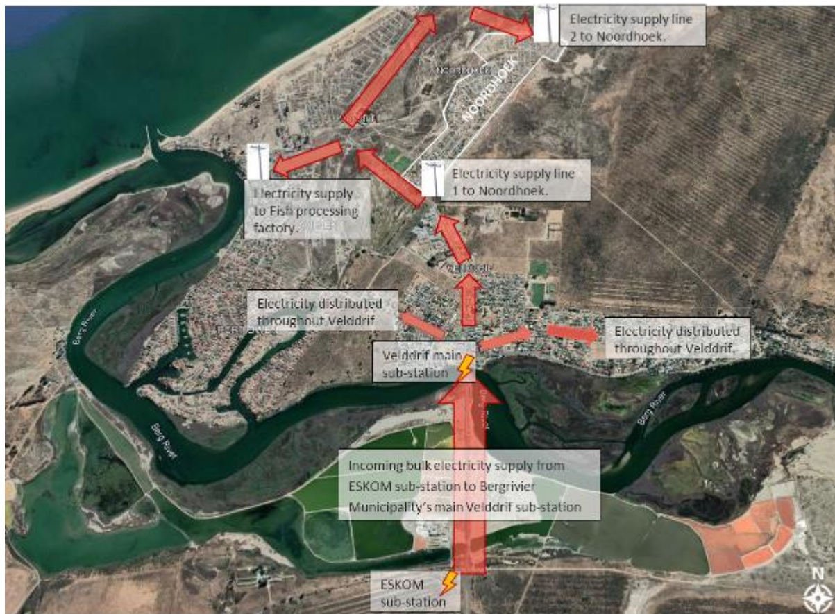
Figure 19: Detail of the electricity supply system to households in Noordhoek. (Source: Author's own on Google Earth base map)
