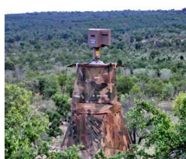
Figure 2: Radar, cameras and information analysis software senses and tracks people entering protected areas.
