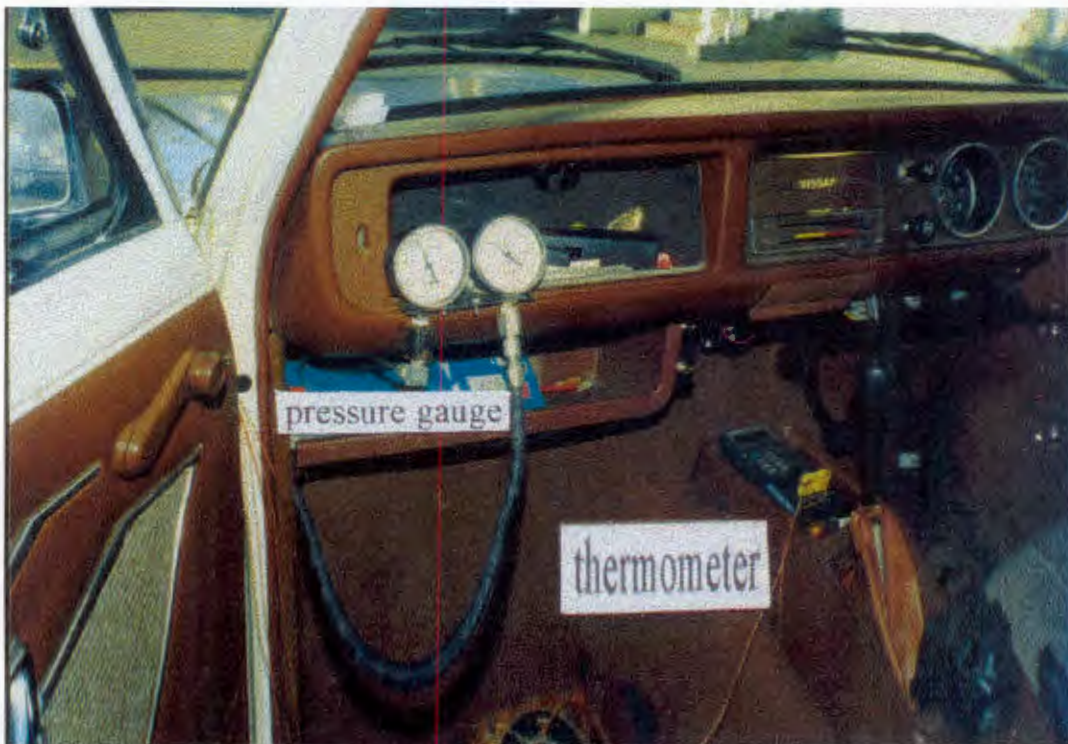
Plate 5-5 Pressure and Temperature Recording from the Cabin.
