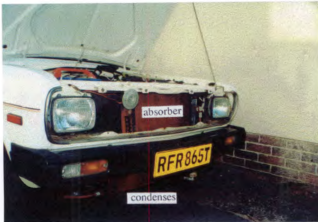
Plate 5-2 The Absorber as Mounted in Front of the Radiator
