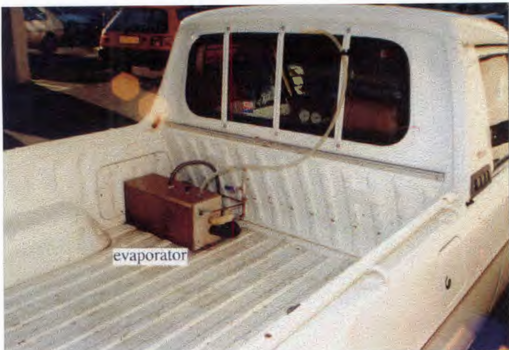
Plate 5-4 The Evaporator Fitted in the Load Box
