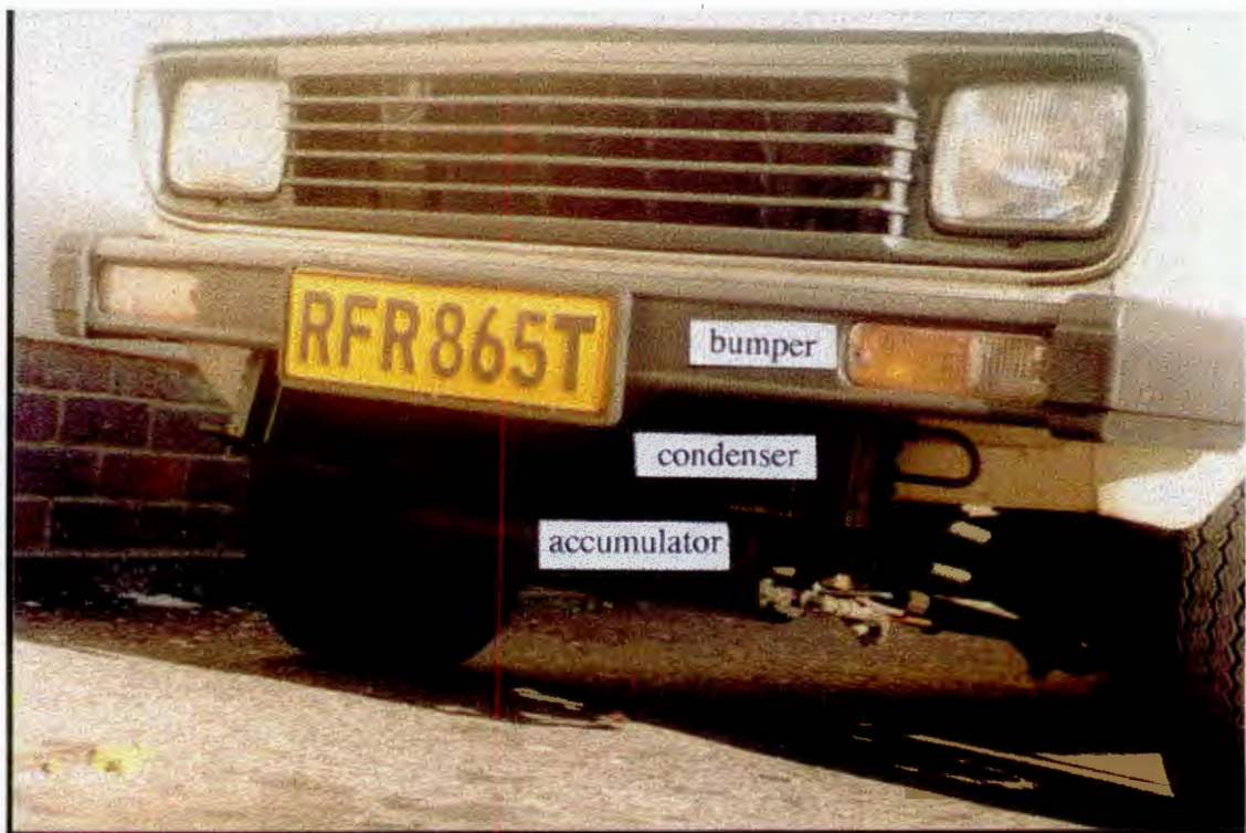
Plate 4-4 The Air-Cooled Condenser in Position
