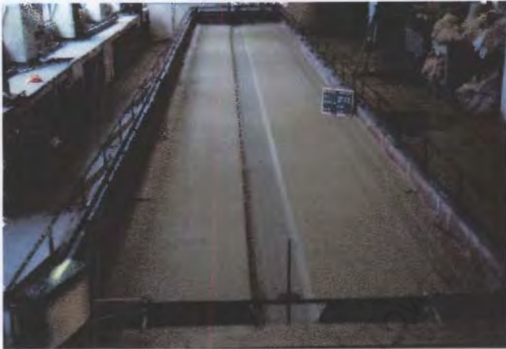
Figure 8.15 : A typical self-formed channel (Babaeyan-Koopaei 1996)
