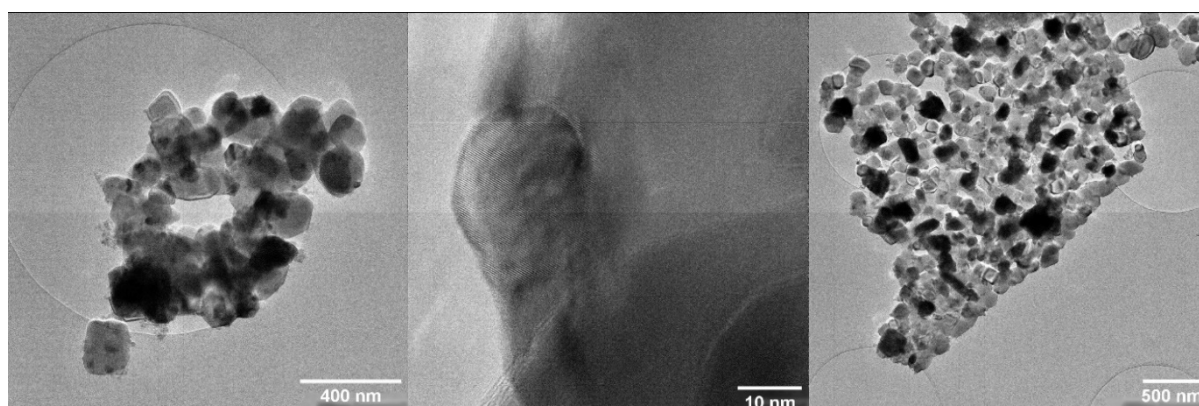
Figure 4.8: TEM images of reduced and steamed catalyst sample (CRS-Cat)
