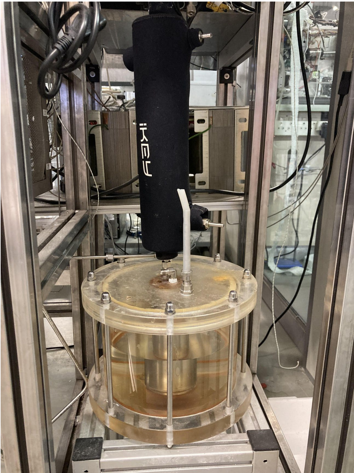
Figure A12.3: Water catch pot and connected chiller
