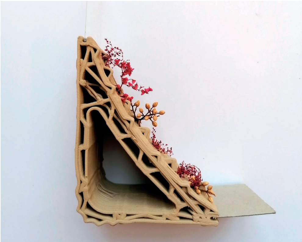
CORNER WALL SECTION - 1 : 25 This portion of the wall hosts services, act as a green wall, and allows for windows dividers to easily slot in
