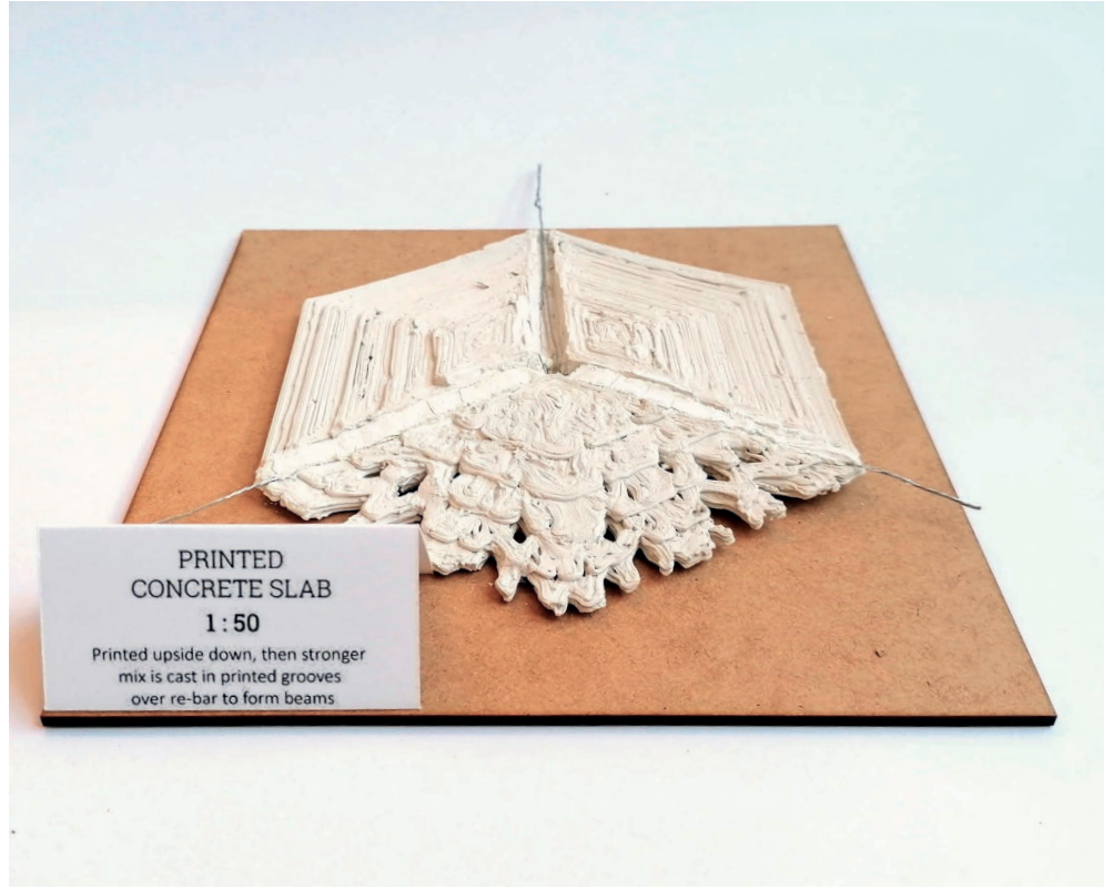
PRINTED CONCRETE SLAB - 1 : 50 Printed upside down, then stronger mix is cast in printed grooves in printed grooves over re-bar
