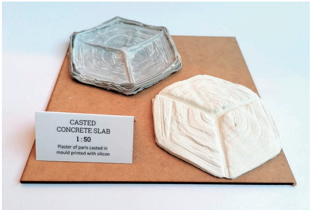
CASTED CONCRETE SLAB - 1 : 50 Plaster of paris cast in mould printed with silicon
