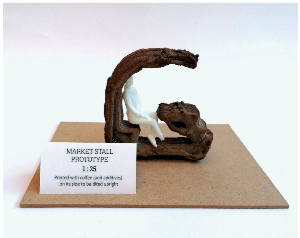
MARKET STALL PROTOTYPE - 1 : 25 Printed with coffee (and additives) on its side to be tilted upright
