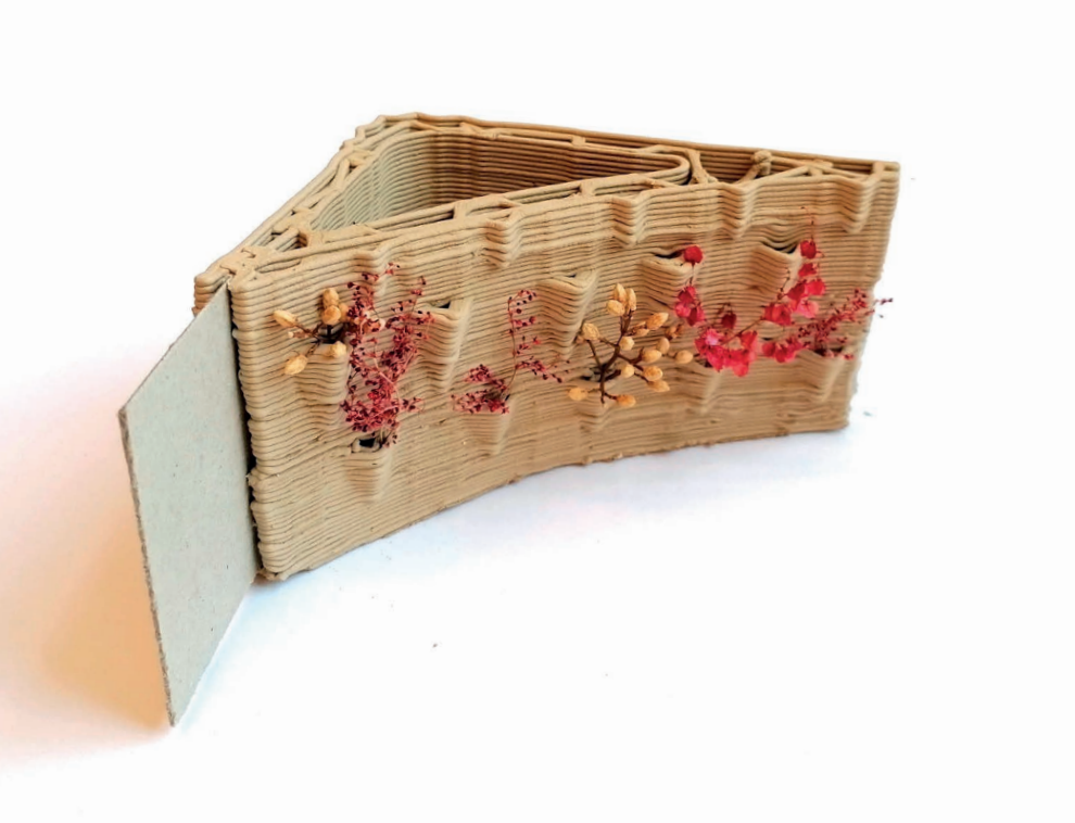
CORNER WALL SECTION - 1 : 25 This portion of the wall hosts services, act as a green wall, and allows for windows dividers to easily slot in
