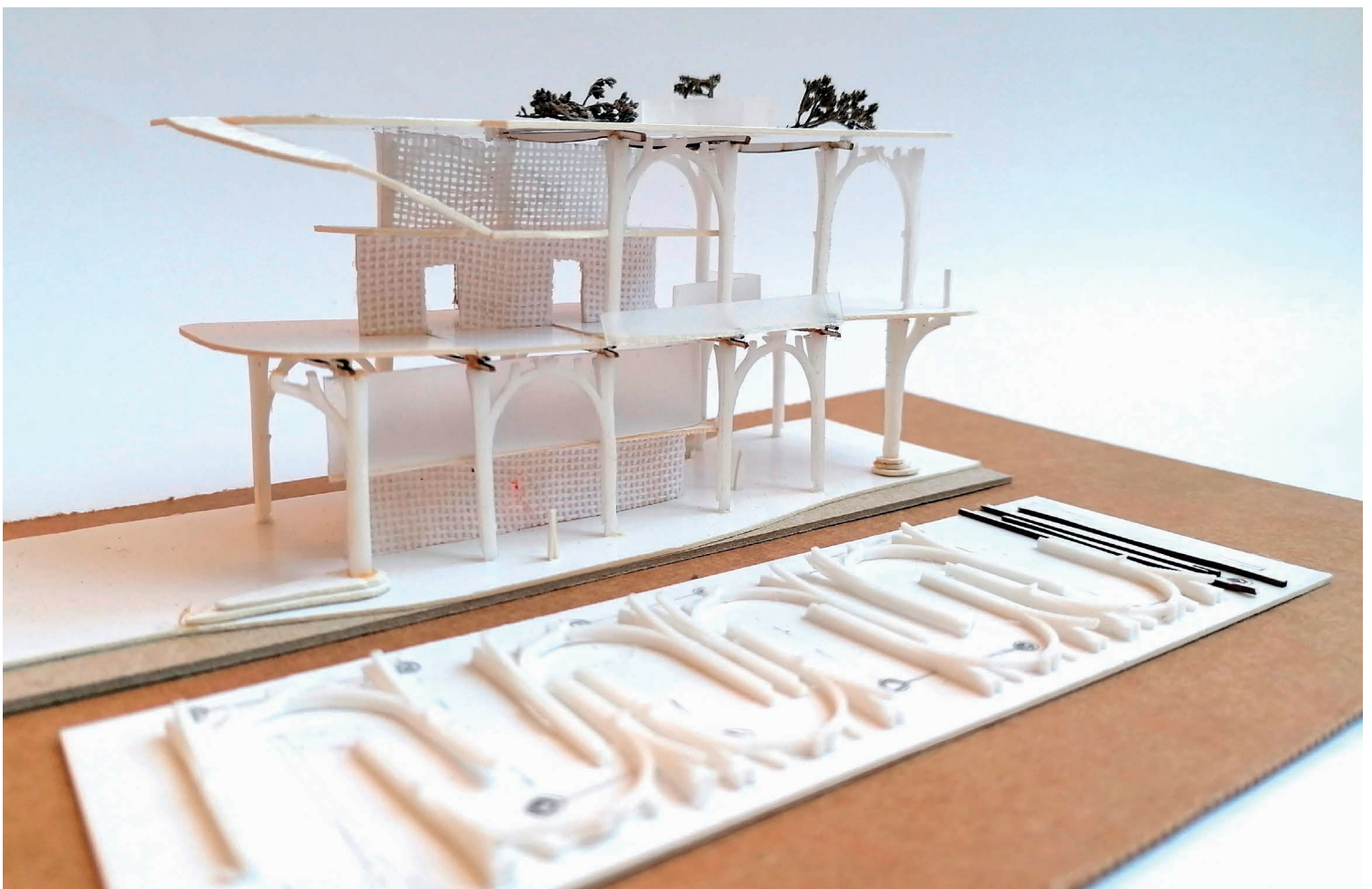
TILT-UP FRAME METHOD - 1 : 200 Explores cost & speed advantages of Tilt-up 3D printed frames for multi-storey housing
