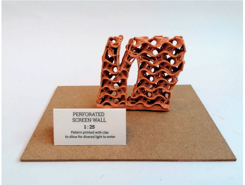
PERFORATED SCREENWALL - 1 : 25 Pattern printed with clay to allow for desired light to enter
