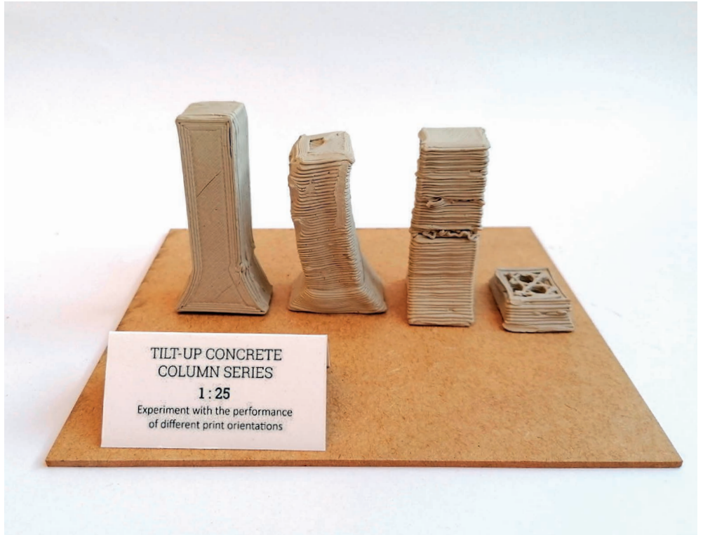
TILT-UP CONCRETE COLUMN SERIES - 1 : 25 Experiment with the performance of different print orientatons
