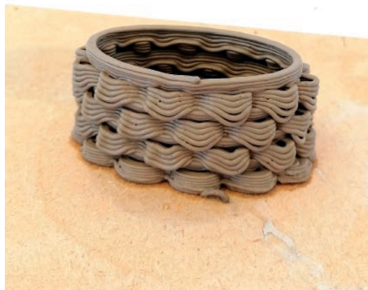
The object was then scaled down to about 5 x 4cm and then successfully reprinted. It took about 15mins.
