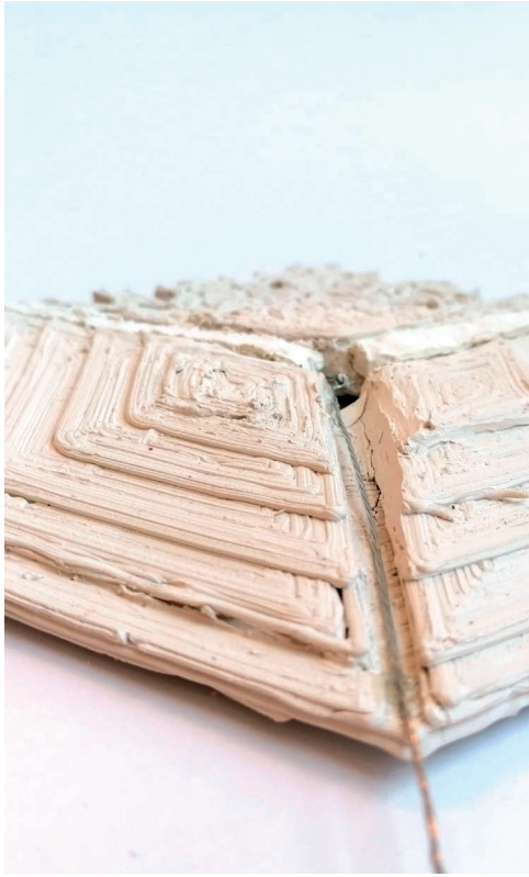
PRINTED CONCRETE SLAB 1 : 50 Printed upside down, then stronger mix is cast in printed grooves over re-bar to form beams
