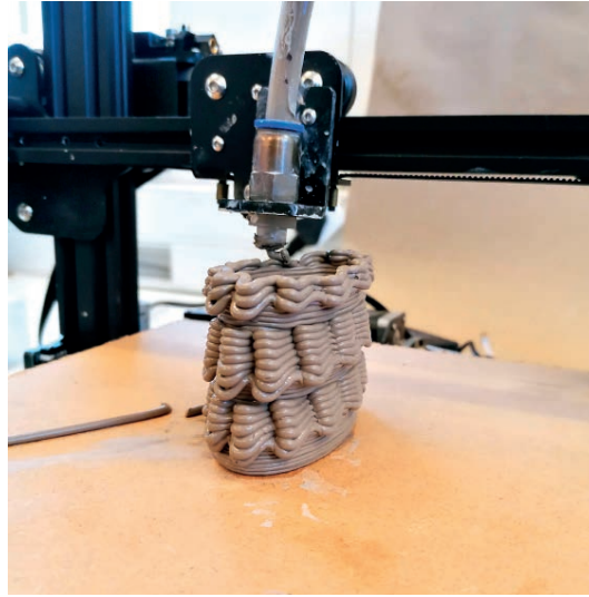
The print in this picture fell over when it reached 8cm because the clay was too wet.
