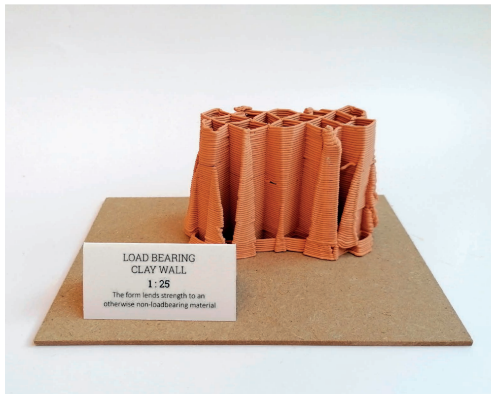
LOAD BEARING CLAYWALL - 1 : 25 The form lends strength to an otherwise non-loadbearing material
