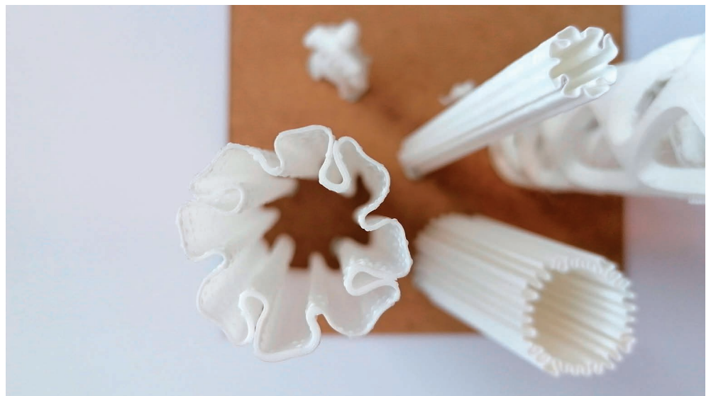
STRUCTURAL COLUMNS - 1 : 50 Explores the strength of the different forms
