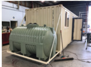
Figure 45: Mobile Decentralized Waste Water System Concept
