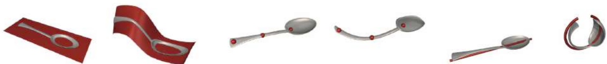
Fig. 19. From left to right: Spatial deformation based on surface, points and curves as dimensions (Gain & Bechmann, 2008)
