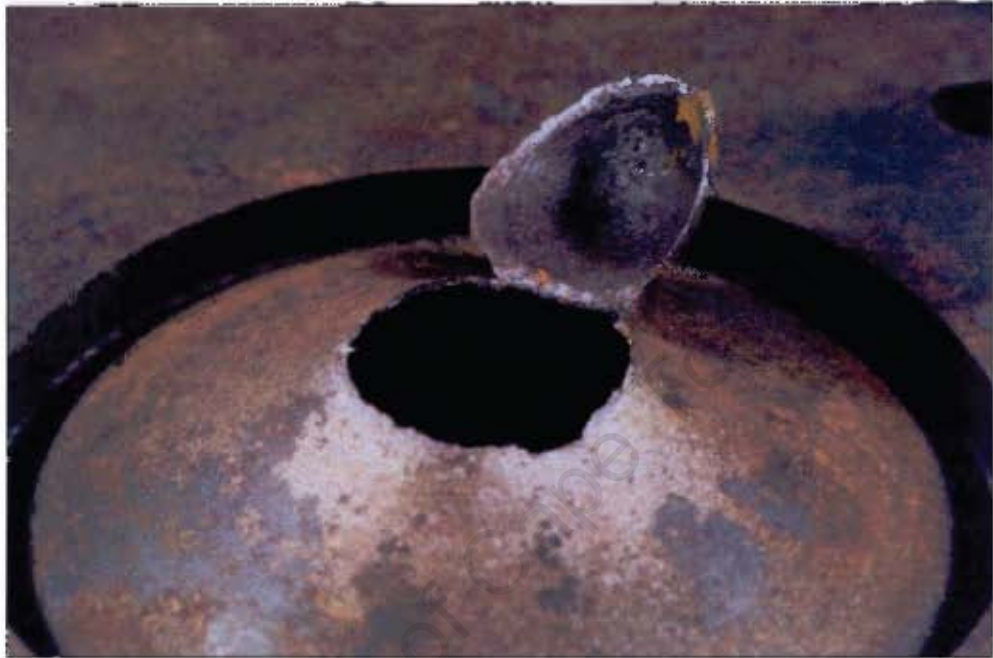
Figure 3.9: 80 % Tearing in the Region of Capping.
