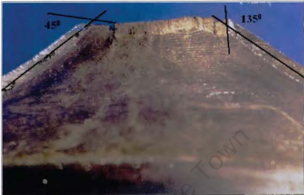
Figure 3.10: Plate Cross Section Showing the Different Angles of Fracture.
