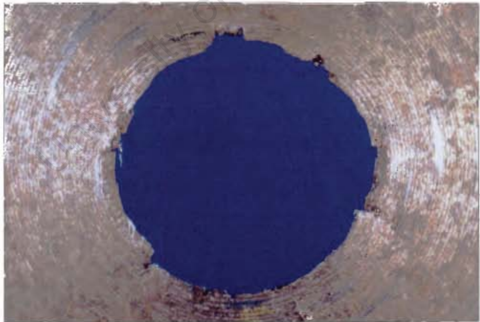
Figure 3.12: A Plate with a Fracture Angle of Mainly 135^{\circ} .
