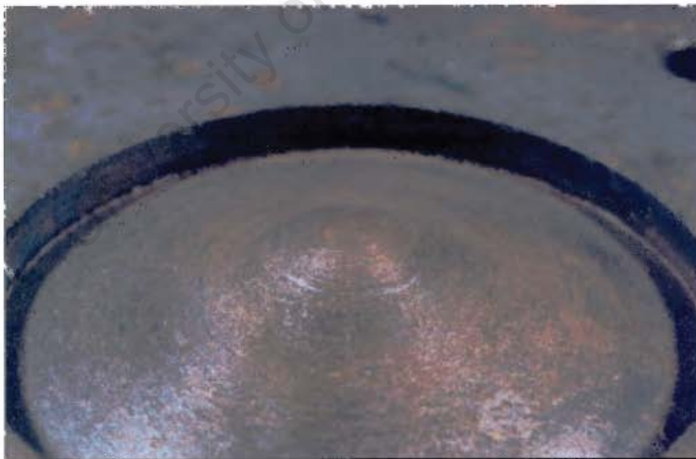
Figure 3.5: A Top View of a Plastically Deformed Plate.
