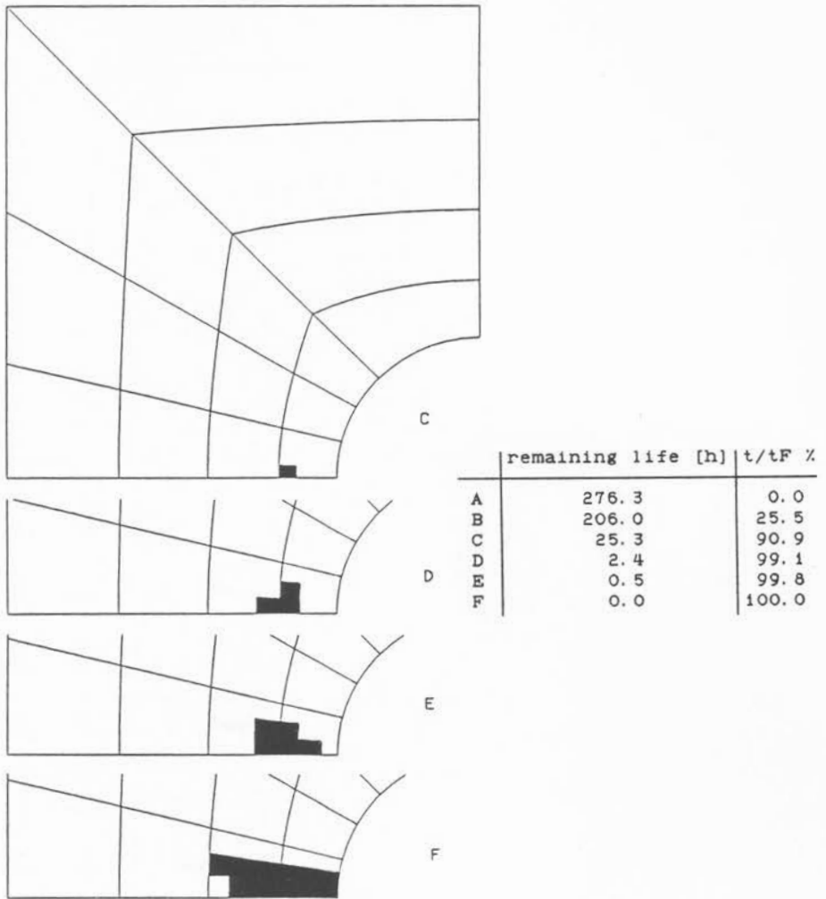
fig. (5.8a) Damage evolution in an axisymmetric tension specimen
