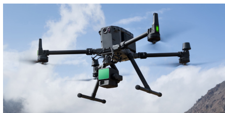
Figure 1.2: DJI Matrice 350 RTK uses the Zenmuse L2 LiDAR to identify any hazard [3].
