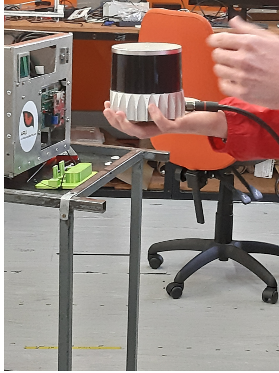
Figure 5.20: Experimental setup in the Mechatronics Lab at UCT, showing Ouster LiDAR (10 Hz) and IMU (100 Hz).
