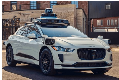
Figure 1.1: The Waymo Driver includes 4 LiDARs that are used for obstacle detection [2].
