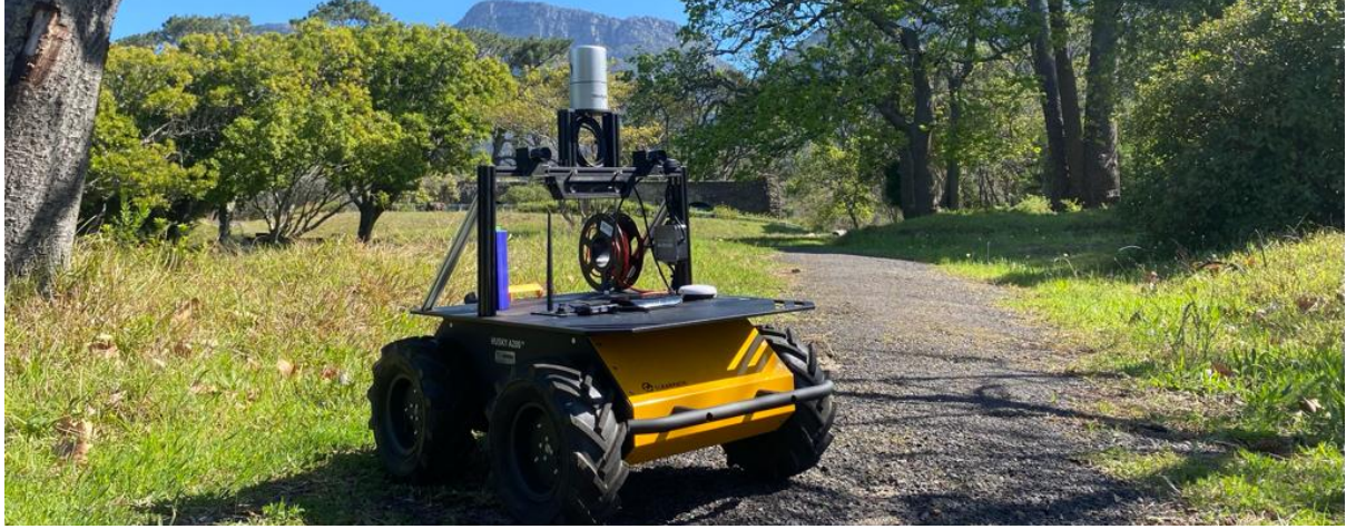
Figure 5.51: Photo of the Clearpath Husky along with sensors used for data collection at the UCT Old Zoo area.
