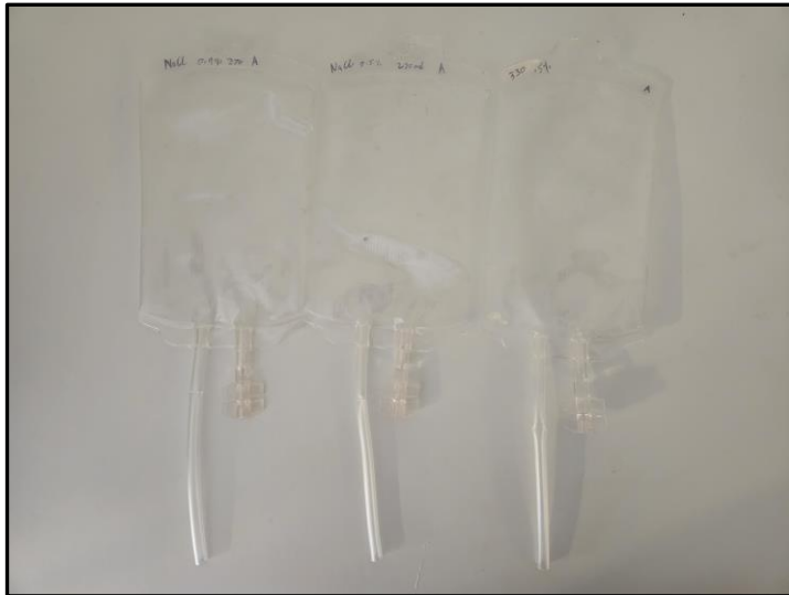
Figure 14 - PVC bags resembling blood bags used during path-finding experiments
