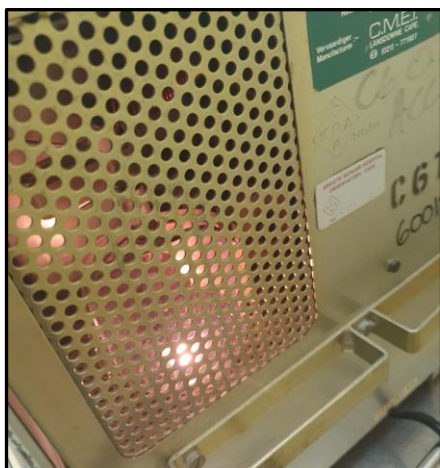
Figure 9 - Taurus 301 valve triode glowing during device operation
