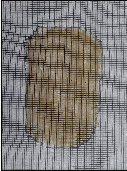
Figure 15 - A roughly rectangular impression, measuring 8x13cm, made by a simulated blood bag used in this study
