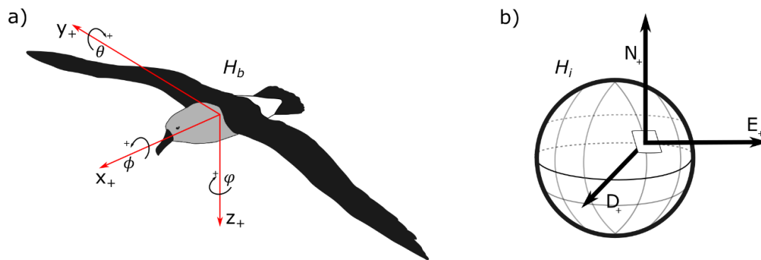
Figure 4.3: a) Body (xyz) coordinate system applied to an albatross, showing the three axes measured by the magnetometers (pitch \theta , roll \phi , and yaw \varphi ) and resultant angles around each axis when compared to b) the north east down (NED) inertial axis system of the reference magnetic field.
