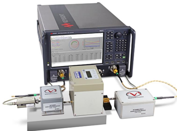
Figure 3.22. A high-accuracy noise figure measurements using the PNA-X series network analyser [55].
