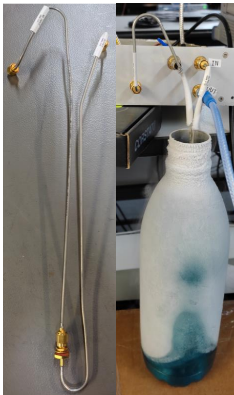
Figure 5.10. The transmission lines and attenuator measured at 77 K.
