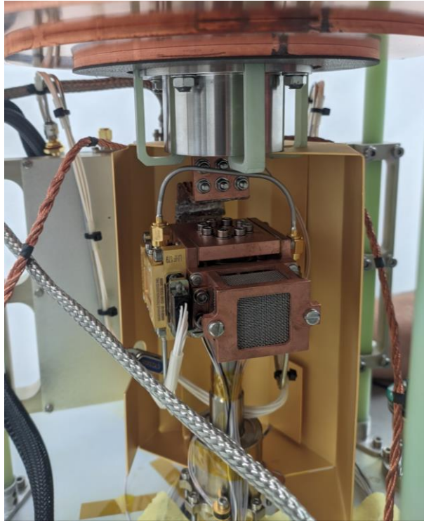
Figure 5.34. The cold attenuator measurement with the AUT on the cold plate.
