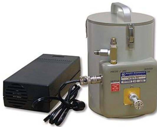
Figure 4.10. Model MT7025J99 cryogenic noise termination and controller [79].
