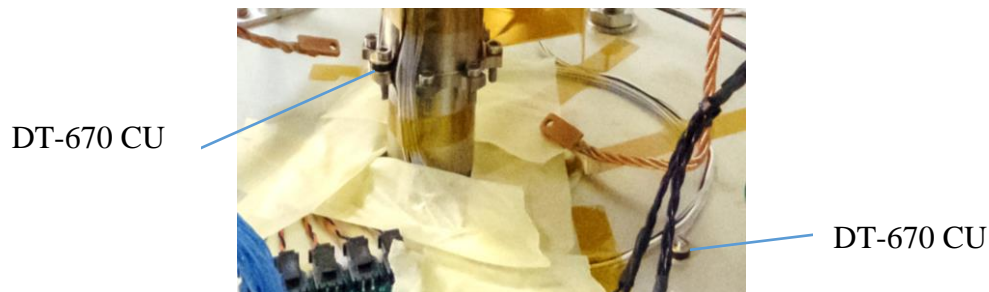
Figure 4.16. The DT-670-CU temperature sensors used in the MeerKAT receiver.
