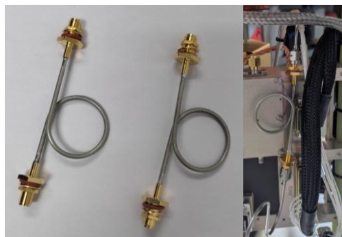
Figure 4.22. The UT-085 jumper cables.
