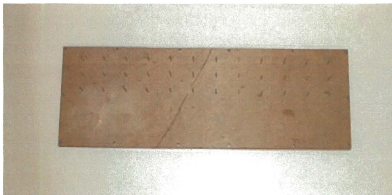
Figure B-16: Tappings on the top face of the rear trailer
