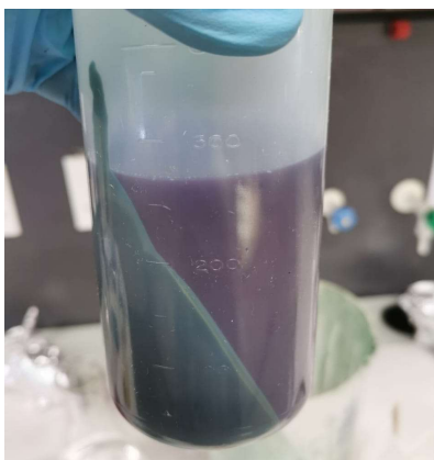
Figure 7: Example of blue supernatant (the crude extract) separated from green biomass pellet after centrifugation.
