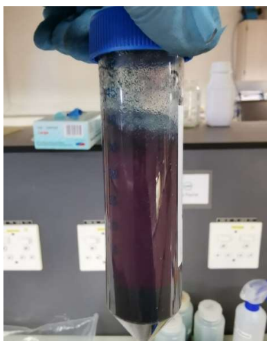
Figure 8: Adsorption step after centrifugation with the blue supernatant above the dark pellet.
