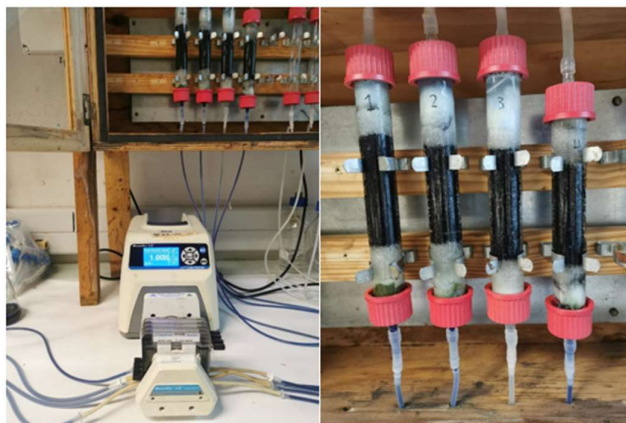
Figure 9: Representation of packed adsorption columns connected to pump with columns seen in more detail.
