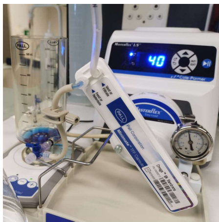
Figure 12: Set up of the ultrafiltration step using a 50 kDa Omega membrane capsule.
