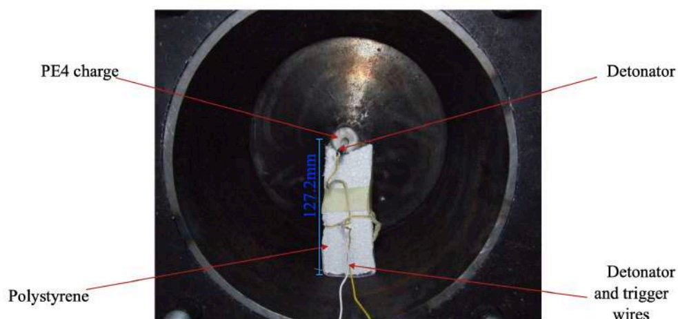
Figure 3.5: Photograph of the placement of the polystyrene stand holding the cylindrical charge
