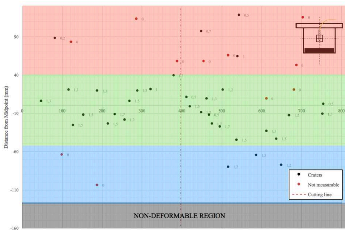
Figure 4.6: Distribution of craters from random-charge test (40 ball bearings, Test #4)
