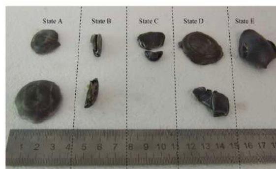
Figure 2.29: Various states of fragments after impact with the rear plate [65]
