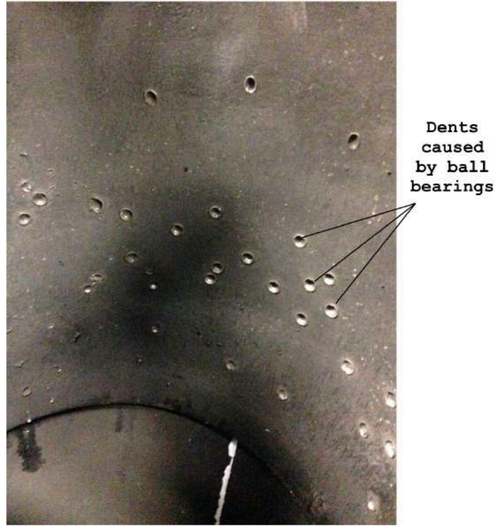
Figure 4.2: Craters on the inner wall of the cylindrical container from test #4 (Random test)
