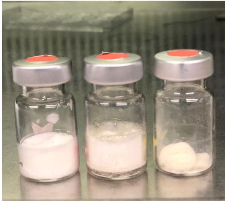
Figure 6-1 Photographic images of freeze dried L. plantarum cells without cryoprotectant, embedded in maltodextrin, and sucrose (from left to right)
