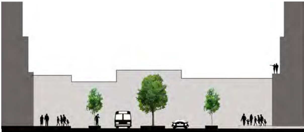
Figure 8.16: Section A-A, illustrating the desired Spatial Environment created by Building Heights (source: Author, 2016).
