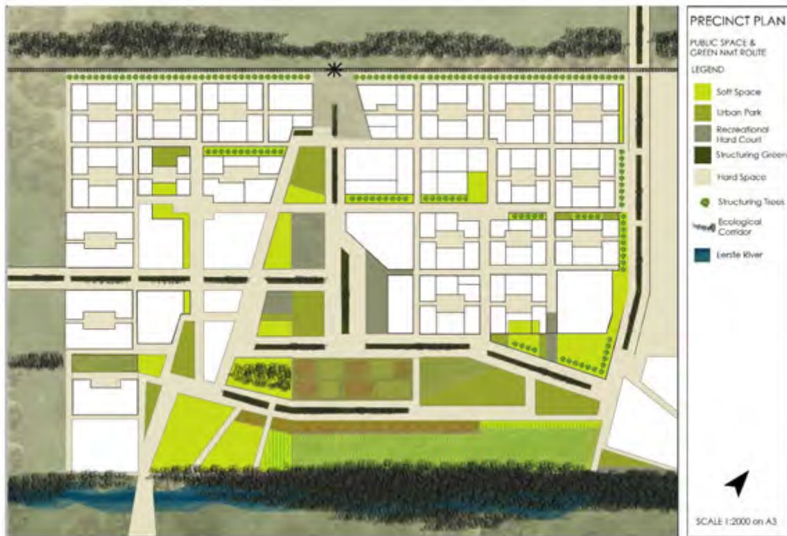
Figure 8.6: Public and Green Space & NMT route network integrating with it (source: Author, 2016).
