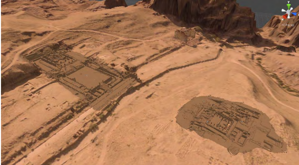
Figure B.2: Example of 3D models automatic placement in Unity if models have been georeferenced to a common co-ordinate system.
