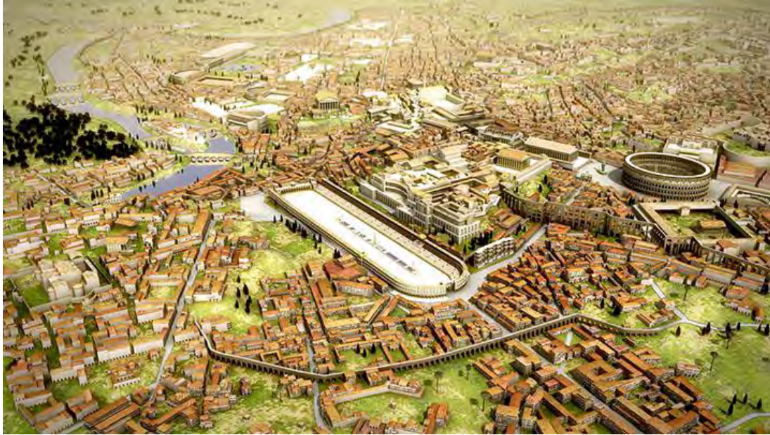
Figure 4.1: Aerial view of the reconstructed city centre of Rome showing buildings on top of a terrain model draped with aerial photography. From (Frischerconsulting, 2013).
