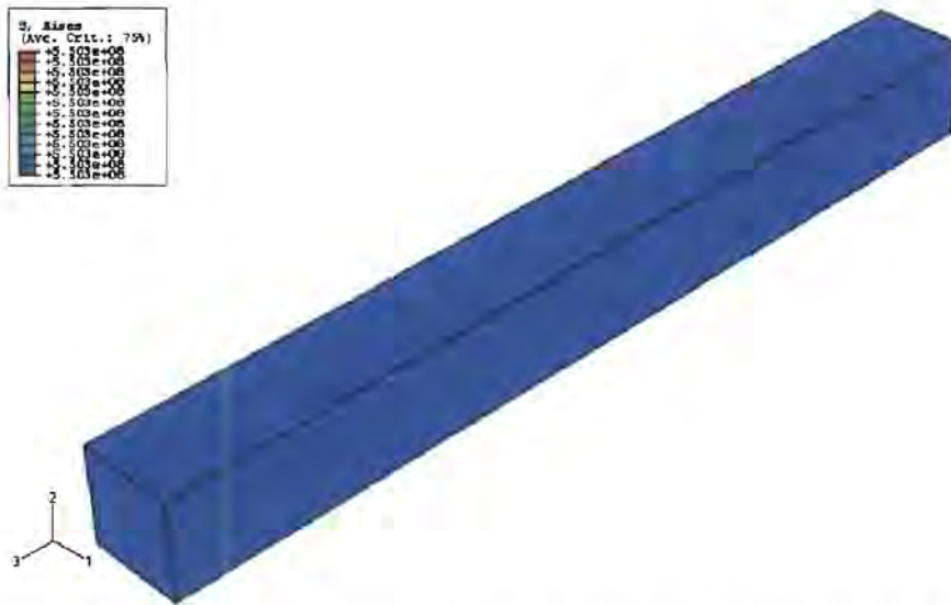
Figure 4.12: Tension - Armco-Iron, 10 m/s using Johnson-Cook VUMAT.
