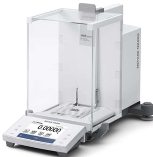
Figure 28: Analytical Balance - Mettler Toledo XS104 (Mettler Toledo, n.d.)
