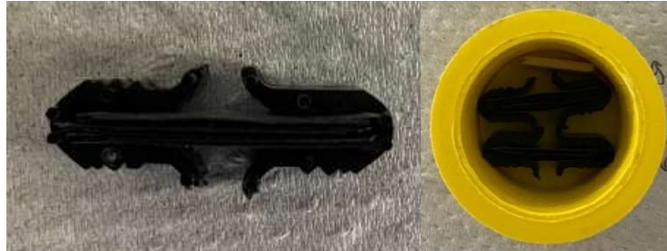
Figure 38: Stacked and clipped sample prior to embedding (left) and mounting cup with samples (right)
