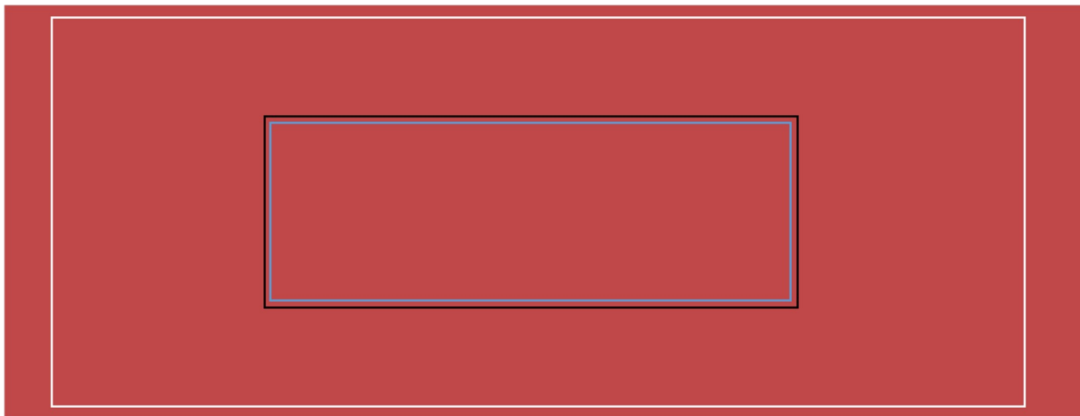
Figure 46: Template for IR MEA features; White - Outer Perimeter of Gasket Frame, Black - CCM Perimeter under Gasket Frame, Blue - AA.
