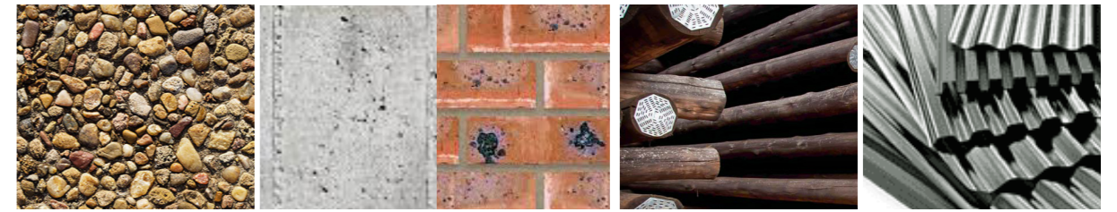
Exposed Aggregate Concrete Old Cape Blend Smooth Brick Treated pine poles Corrugated iron sheets
