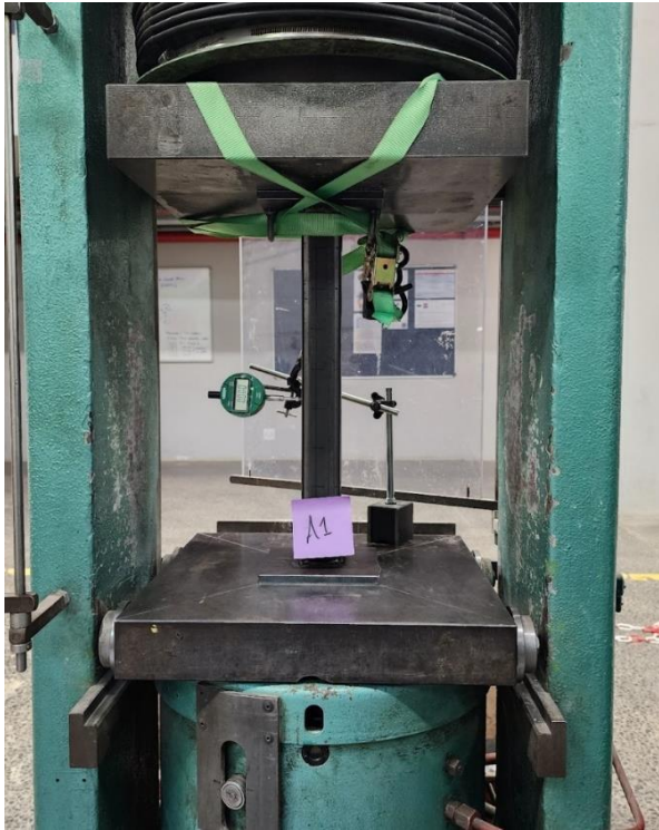
Figure 3-8 Specimen A1 before testing
