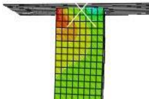
Figure 5-1 Stress concentrations at support (off-centre damage)
