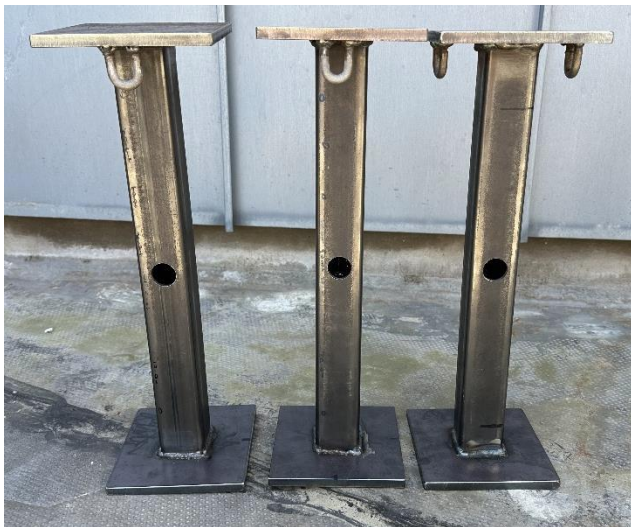
(b) Damaged Specimens (Type B)
