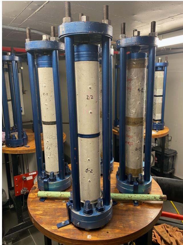
Figure 3-4: Set-up apparatus for compressive creep test
