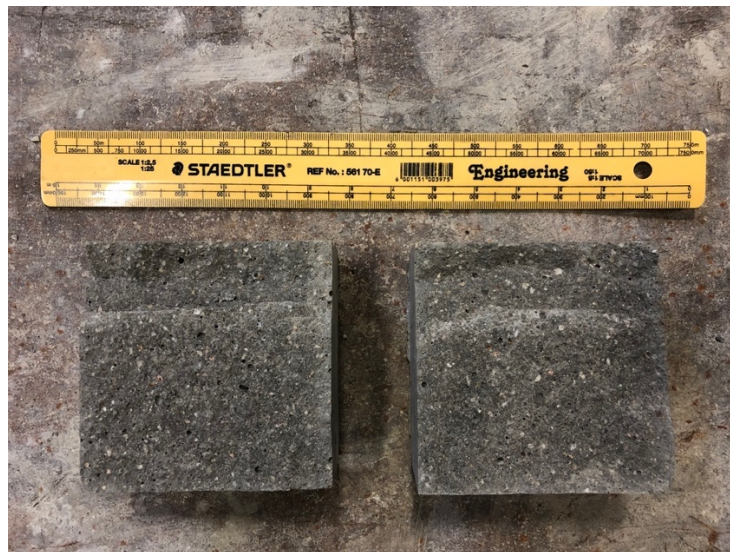
Figure 4-5: Split specimen of HS concrete tested for tensile splitting strength at 1 day
