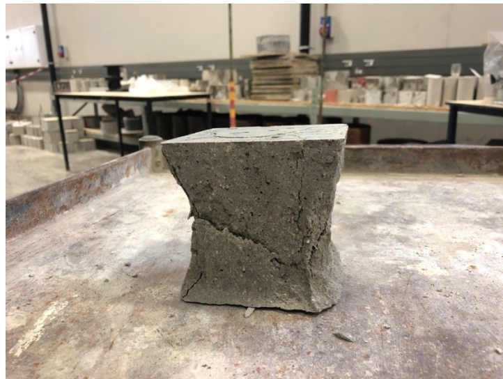
Figure 4-1: Failure mode for PMRM specimen tested for compressive strength at 1 day
