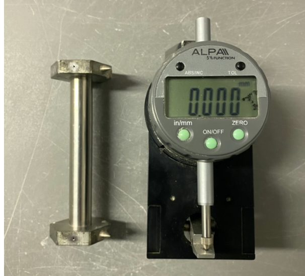
Figure 3-3: Reference bar (left) and strain gauge extensometer (right)
