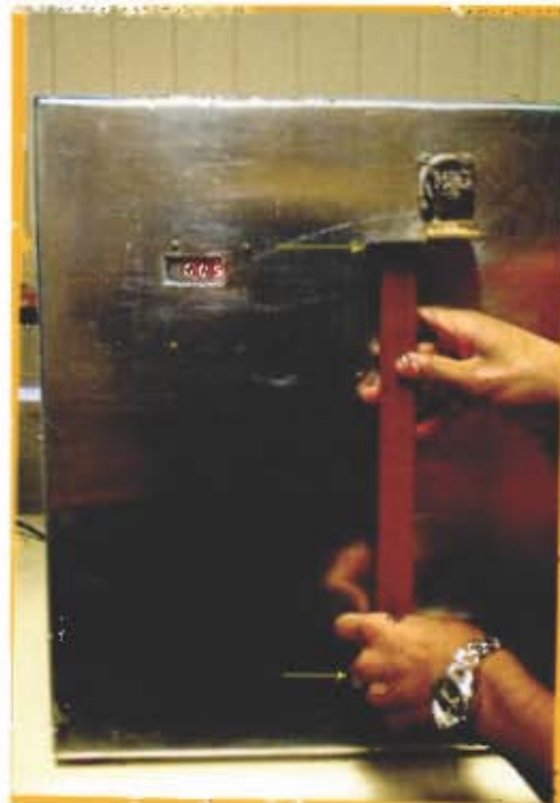
Figure 4.16 Method of Mounting Waveguide Filled with Mineral Sand
