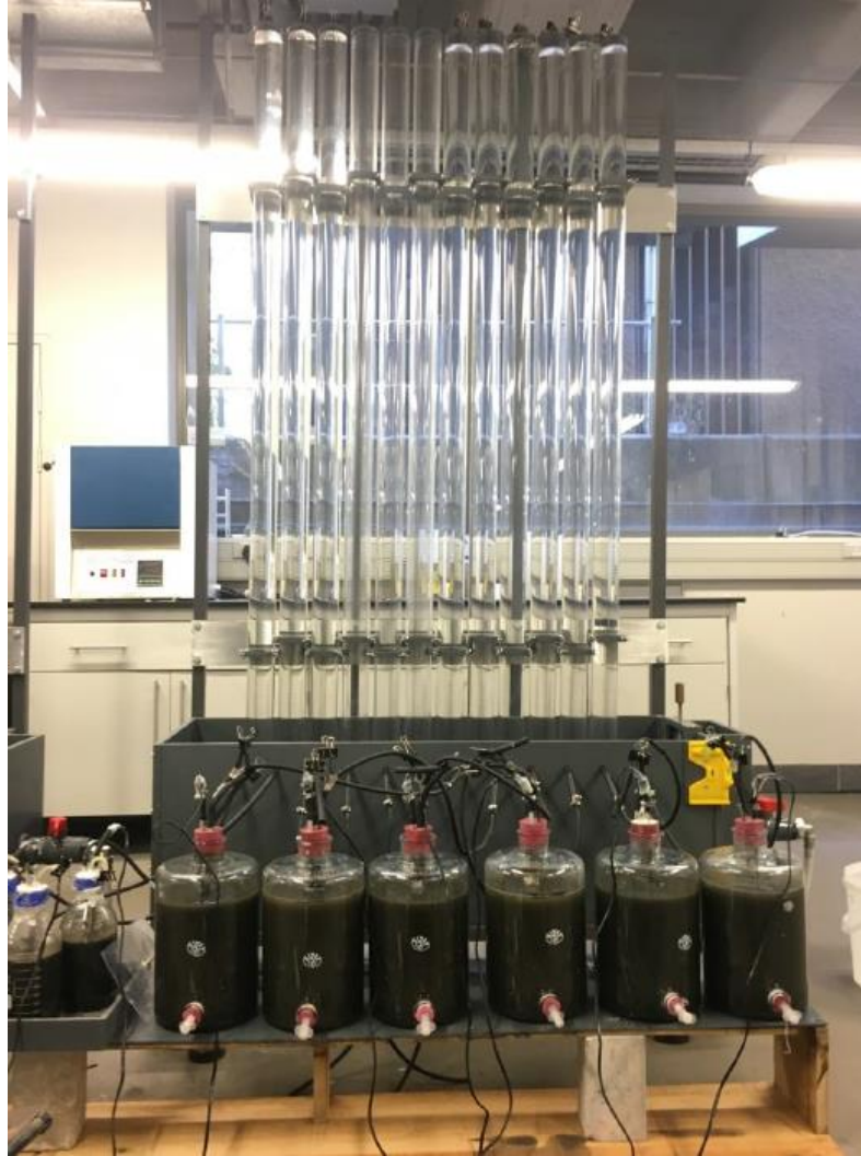
Figure 2.12: Typical ABMP set-up with gas displacement columns
