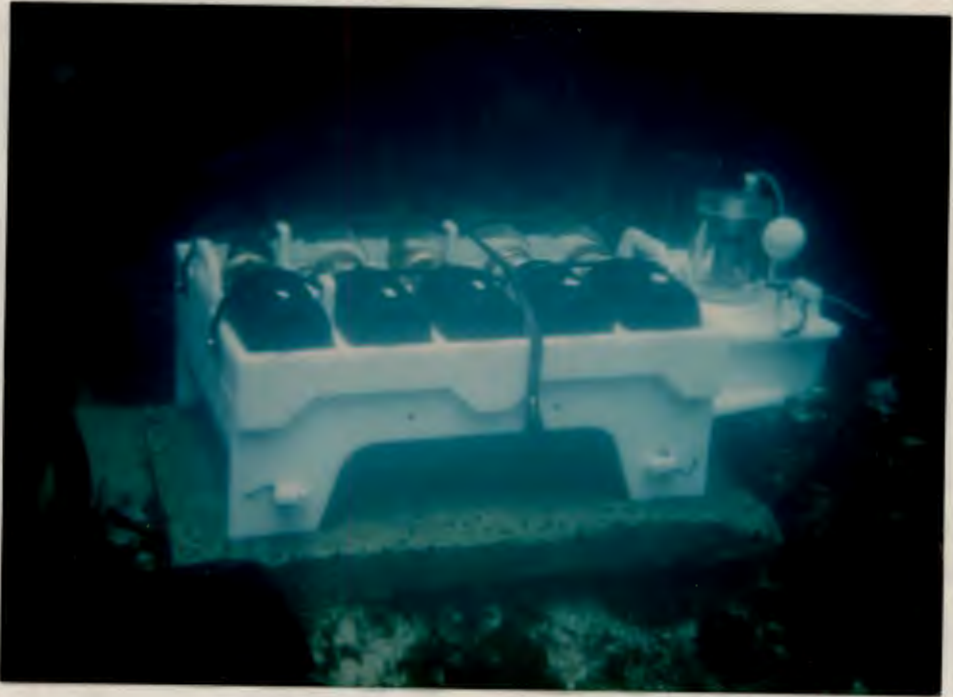
Plate 3: Light and dark bottle incubation apparatus used for in situ photosynthesis measurements on site at Oudekraal.
