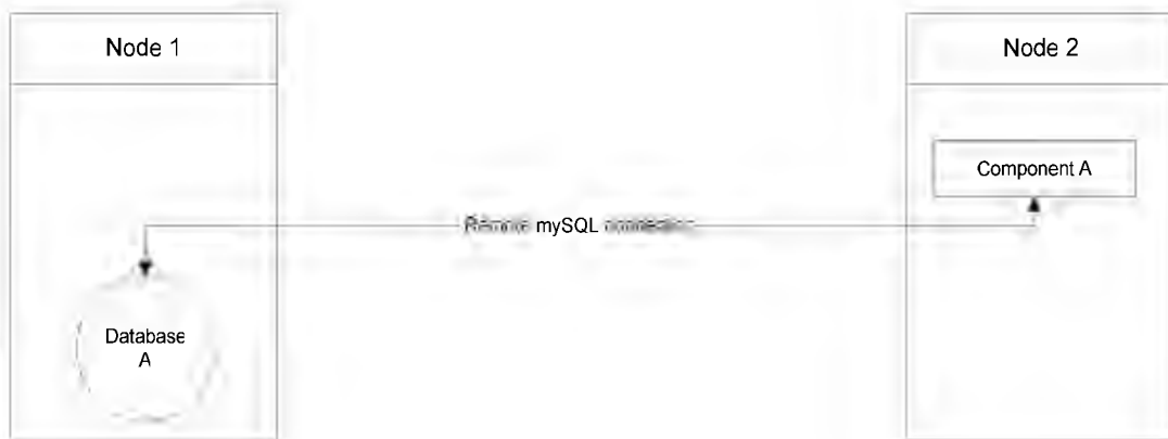
Figure 9: Nodes after component A has been migrated from Node 1 to Node 2. Component A is still using the database which resides on the original node.
