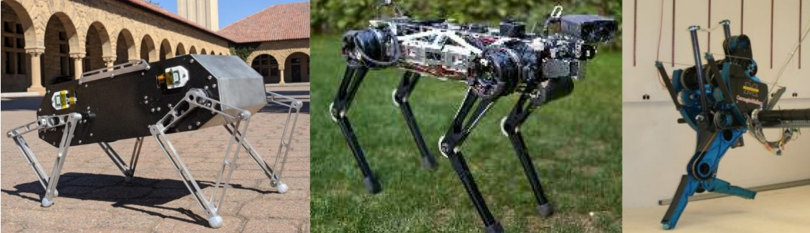
Figure 4: Legged robots which used Force control techniques to obtain desired locomotive tasks. The Stanford Doggo is on the left [20], MIT Mini Cheetah in the centre [46], and MABEL on the right [45].
