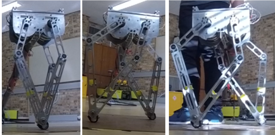
Figure 46: Images of the 0.5 m/s (left), 1.5 m/s (centre), and 4.0 m/s (right) final deceleration stance.
