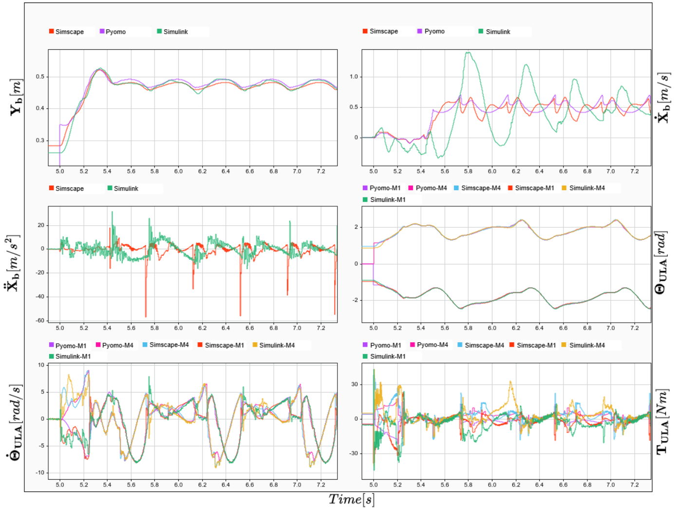
Figure 42: Snapshot of the 0.5 m/s walk, displaying Pyomo, Simscape, and Simulink curves. Between time-stamp t = 5 seconds and t = 5.6 seconds highlights the acceleration trajectories.
