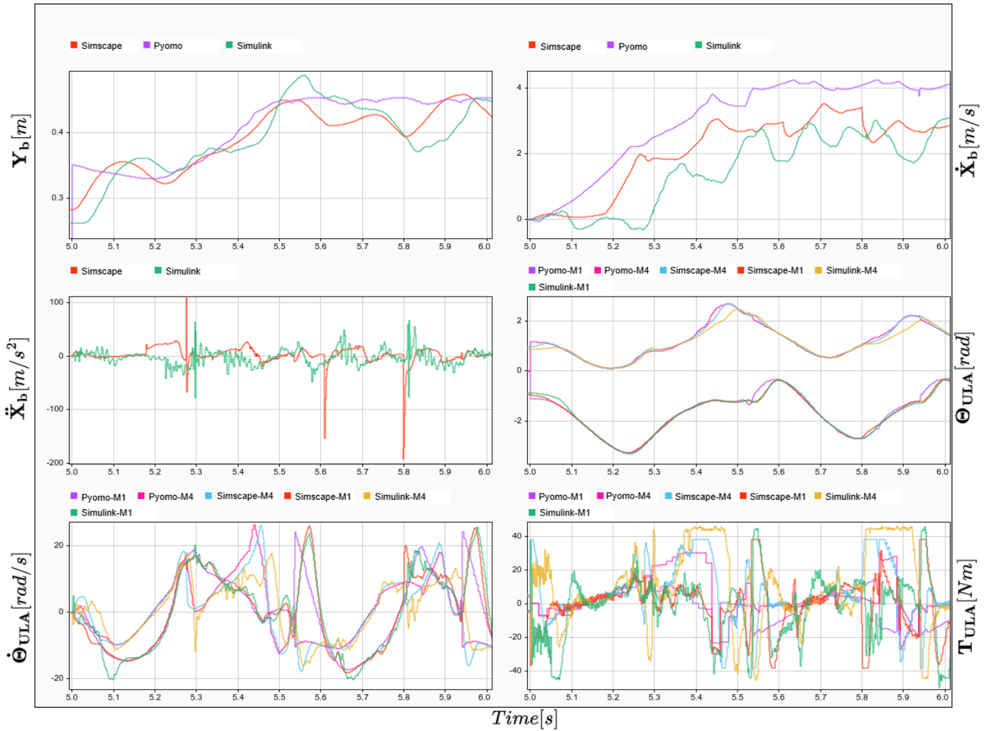
Figure 52: Snapshot of the 4.0 m/s results, displaying Pyomo, Simscape and Simulink curves. Between time-stamp t = 5 seconds and t = 5.5 seconds highlights the acceleration trajectories.
