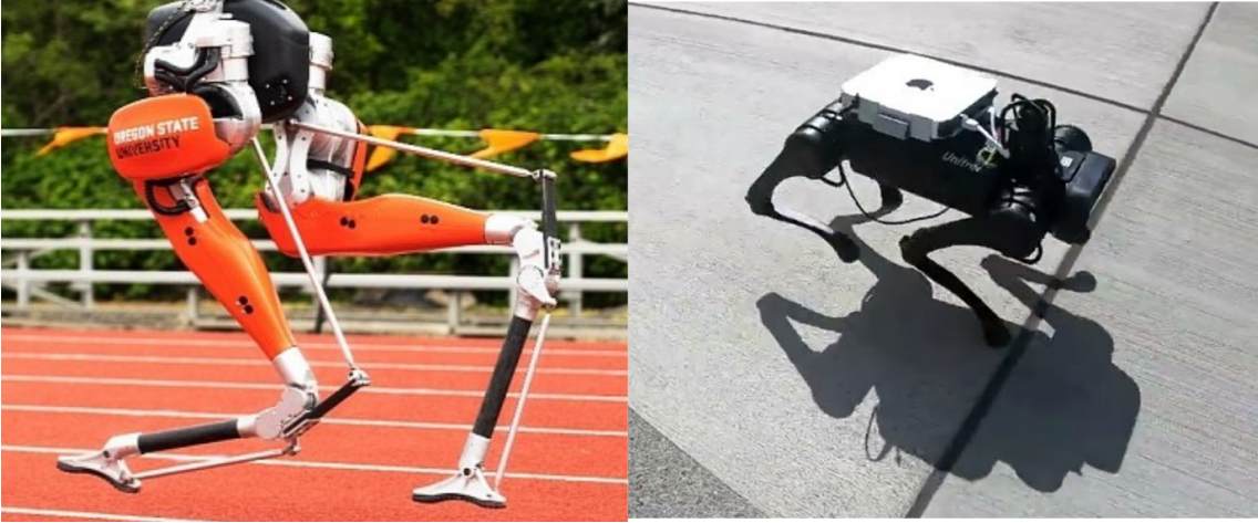
Figure 6: Cassie [10] (left) and Unitree [13] (right) use RL to achieve their desired locomotive tasks.
