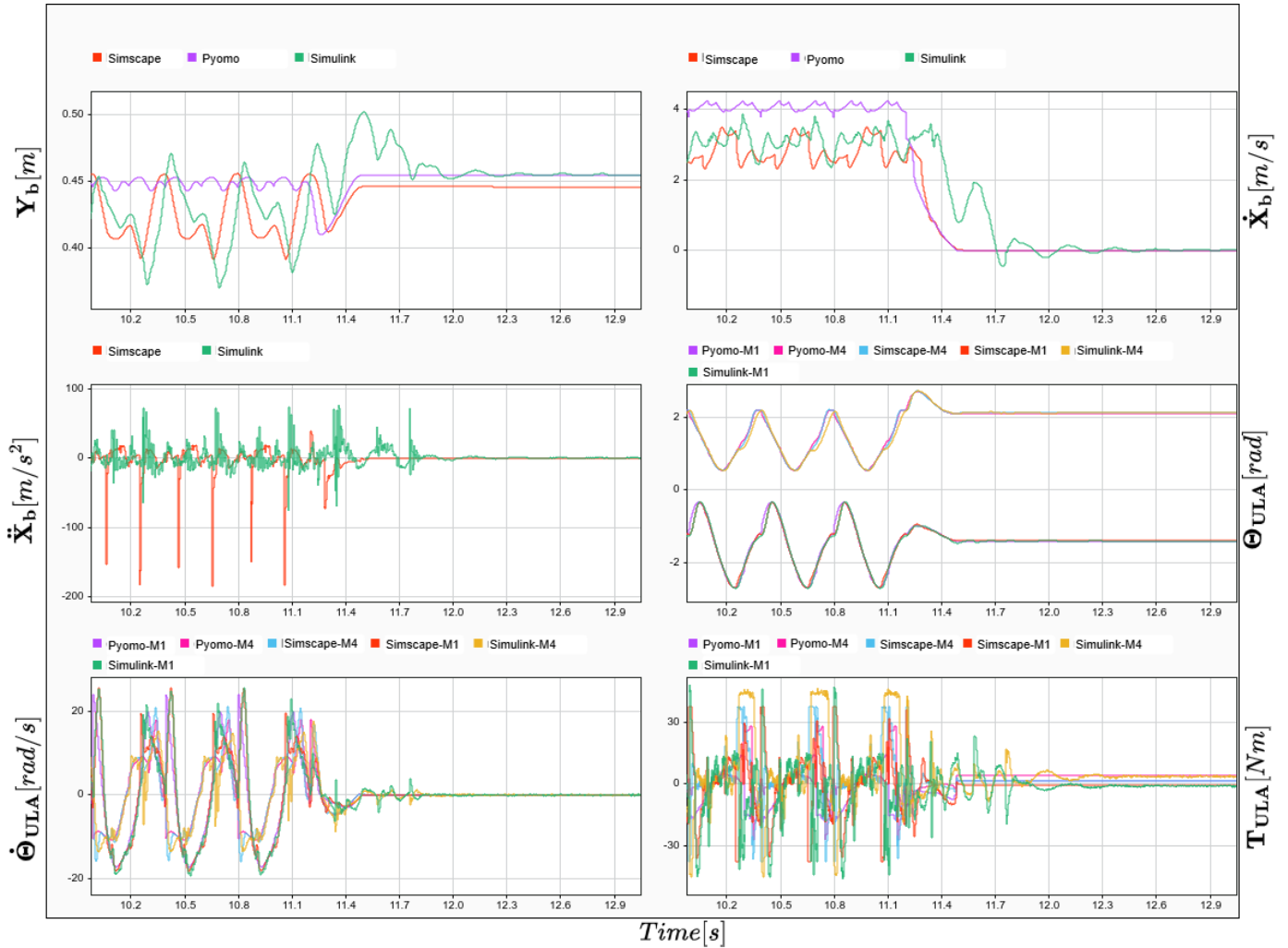
Figure 54: Snapshot of the 4.0 m/s top speed simulation, displaying Pyomo, Simscape, and Simulink curves when the robot decelerates.
