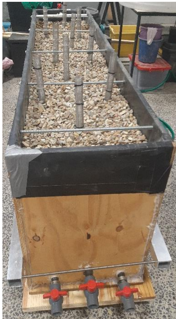
Figure 5.5: Complete pilot biofilter
