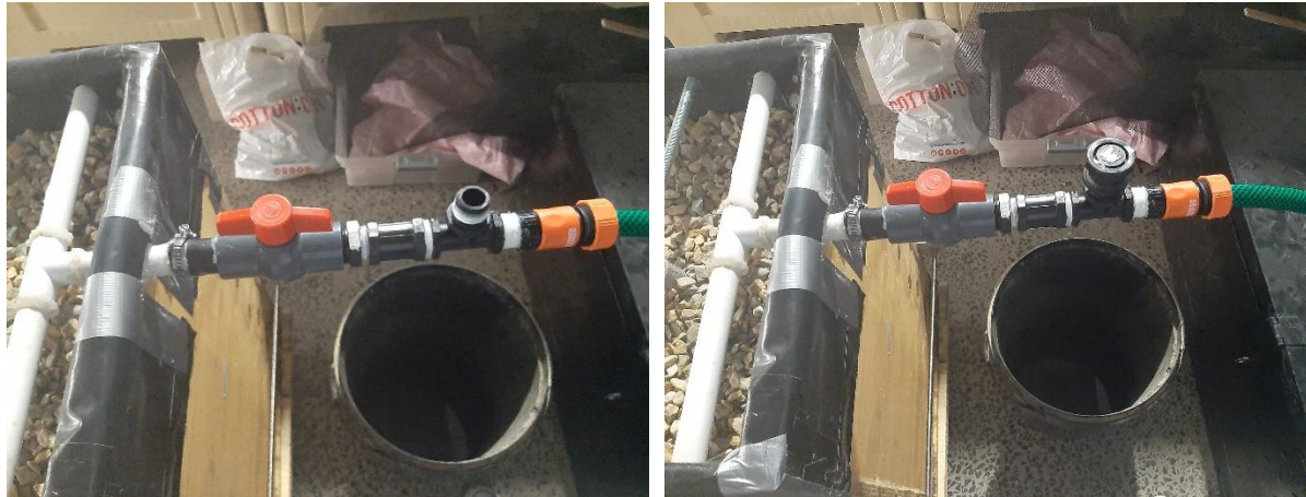
Figure 5.7: Inlet for tracer injection (inlet opened in left image and closed in right image).
